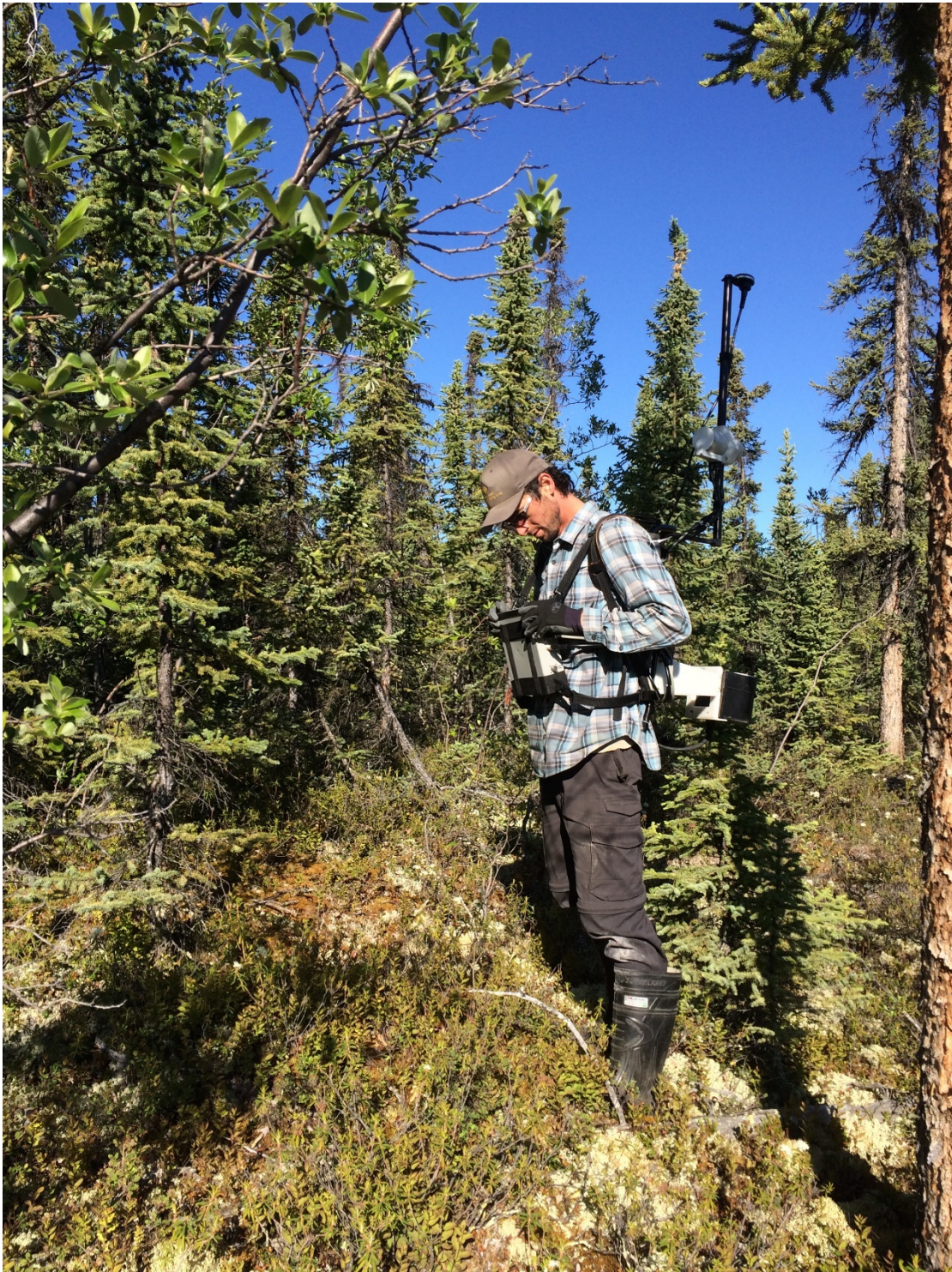
Figure 4 Overhauser walk-mag GSM-19 magnetometer rover backpack mounted unit with GPS in action at the Carmack Copper Project (this unit also has a modular VLF sensor, which was not used in the program).
