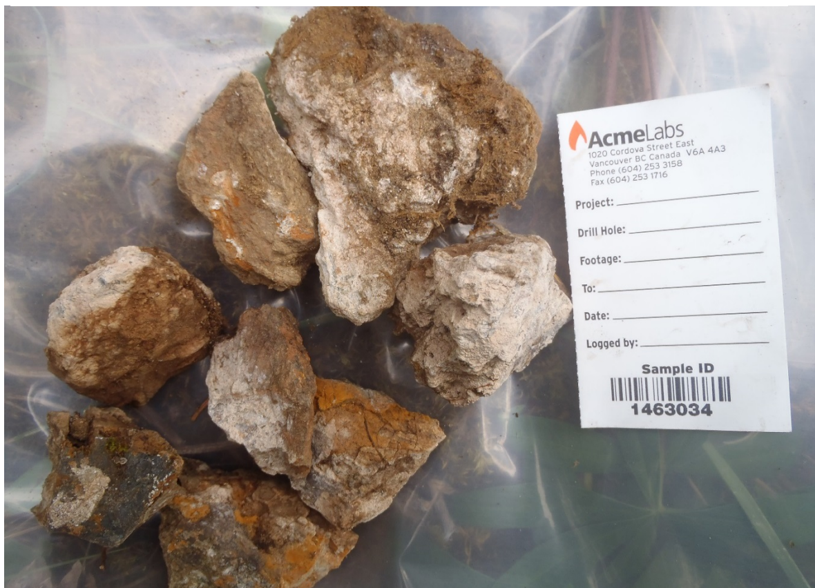
Figure 5: Contact breccia elevated in Cu (228 PPM)
