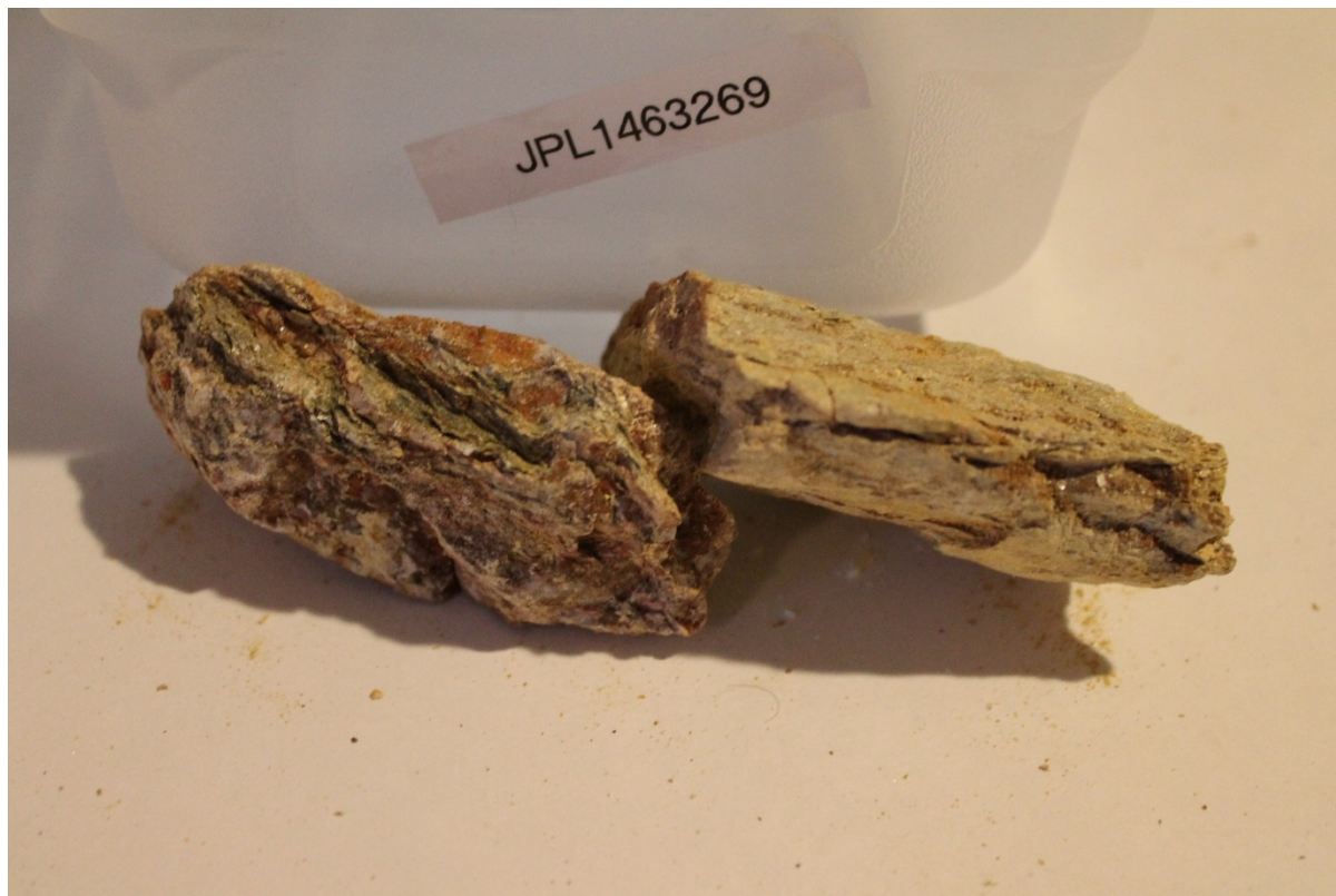
Figure 19: Rocks with talc and elevated in Cu-Pb-Zn-Au-Ag. Soapy feel. Possible footwall alteration zone?
