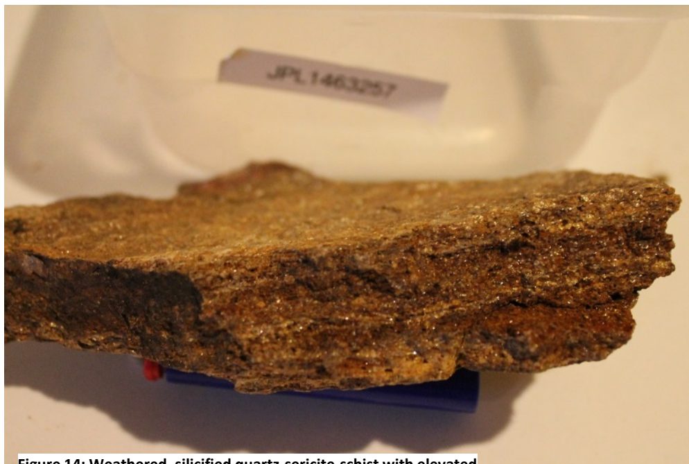
Figure 14: Weathered, silicified quartz-sericite-schist with elevated Cu (163 PPM), Pb (3332 PPM), Zn (682 PPM)
