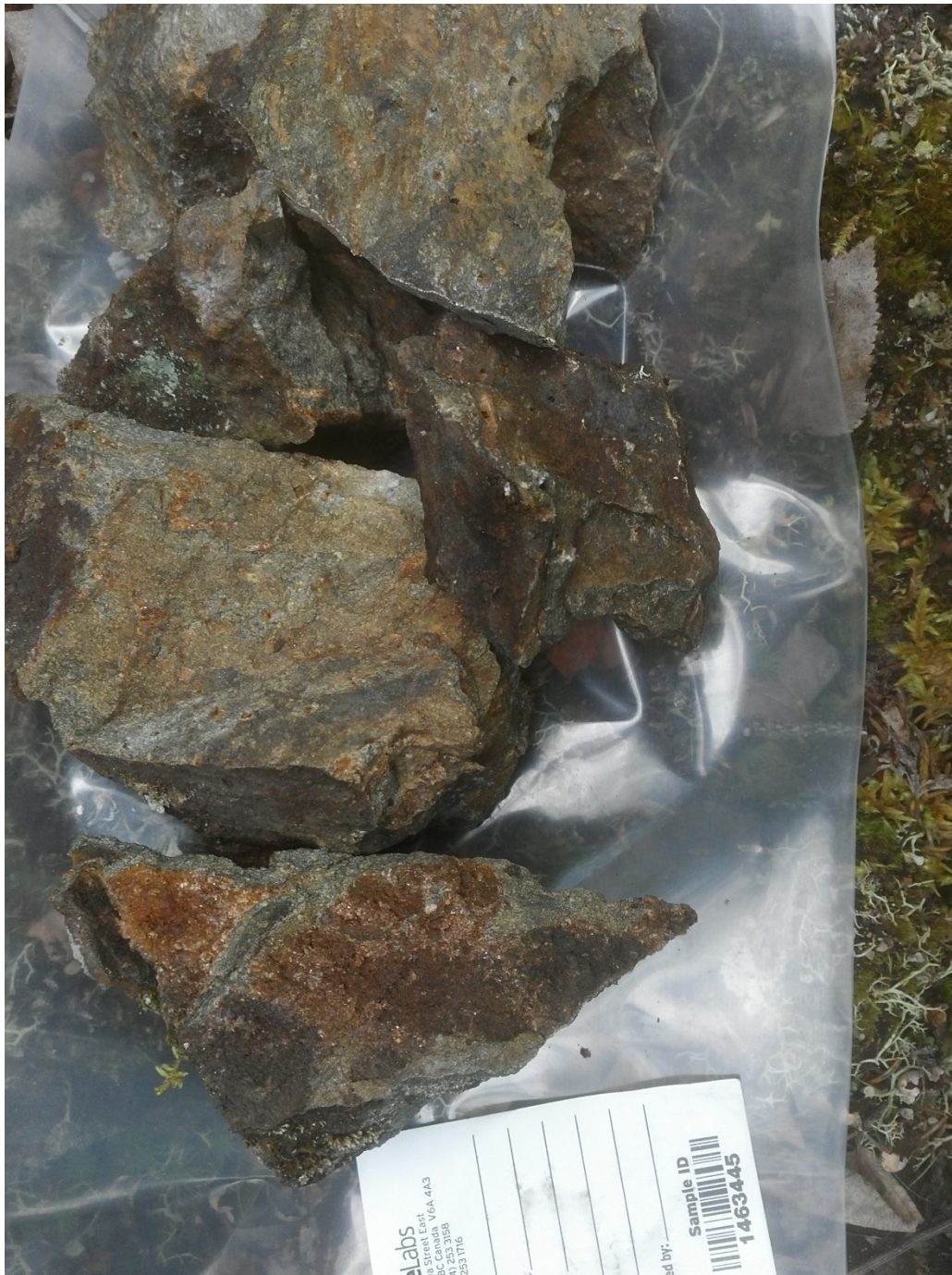
Figure 22: Mafic basalt flow? Much weathered out py vugs. Slightly foliated.
