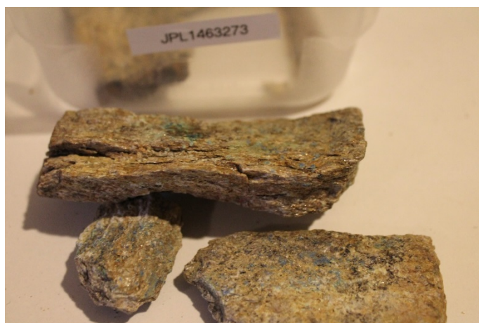
Figure 12: Schist with 0.3% Cu, visible calcite, and surprisingly low in Pb and Zn. Meta-rhyolite dyke syngenetic with surrounding meta-tuff?
