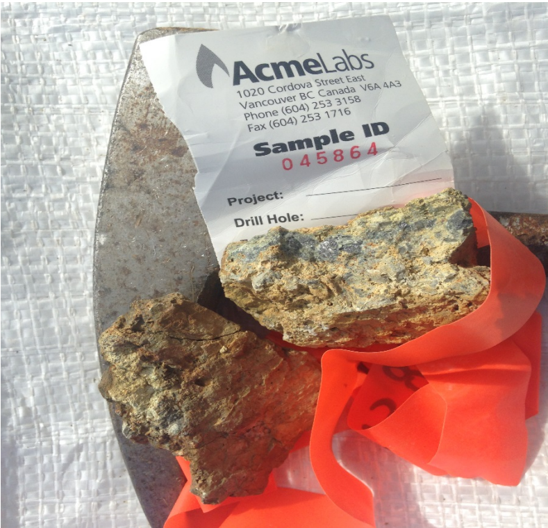
FIGURE 18 MASSIVE ARSENOPYRITE AND QUARTZ VEIN MATERIAL FROM LOWER TREADWELL ADIT DUMP (9.0 G/T GOLD)
