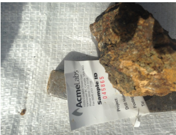
FIGURE 16 TREADWELL ADIT DUMP ROCK WITH ROCK FRAGMENTS CEMENTED IN FAULT GOUGE
