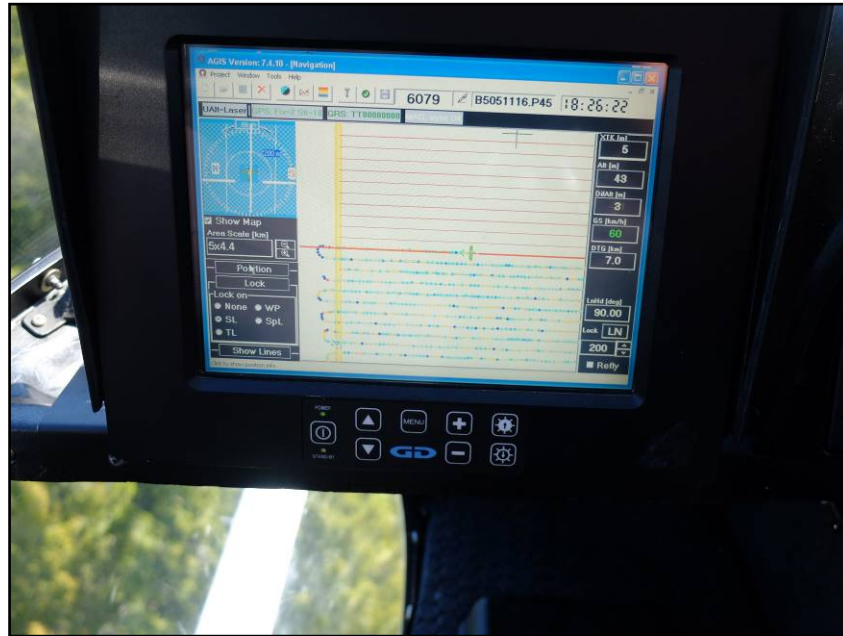
Figure 11: AGIS operator display installed in the Eurocopter AS350, with screen displaying real time flight line recording and navigation parameters.
