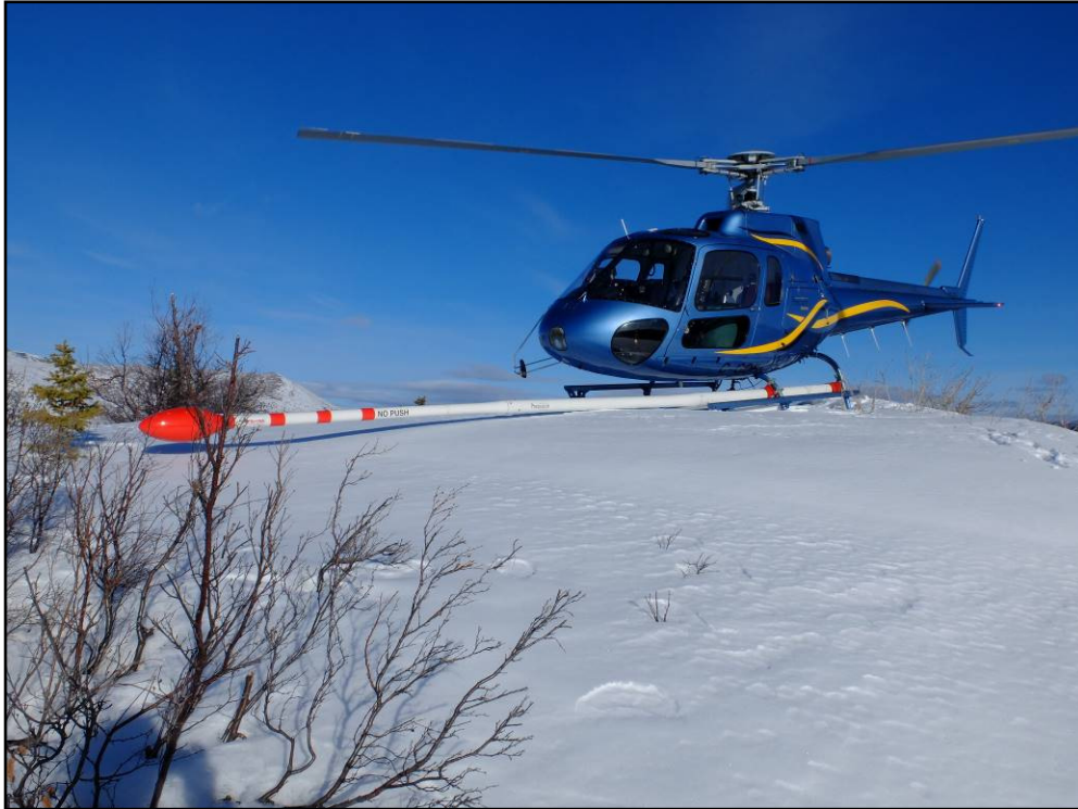
Figure 10: Eurocopter AS350 helicopter equipped with mag stinger for magnetic data acquisition, and internal spectrometer crystals for radiometric data acquisition.
