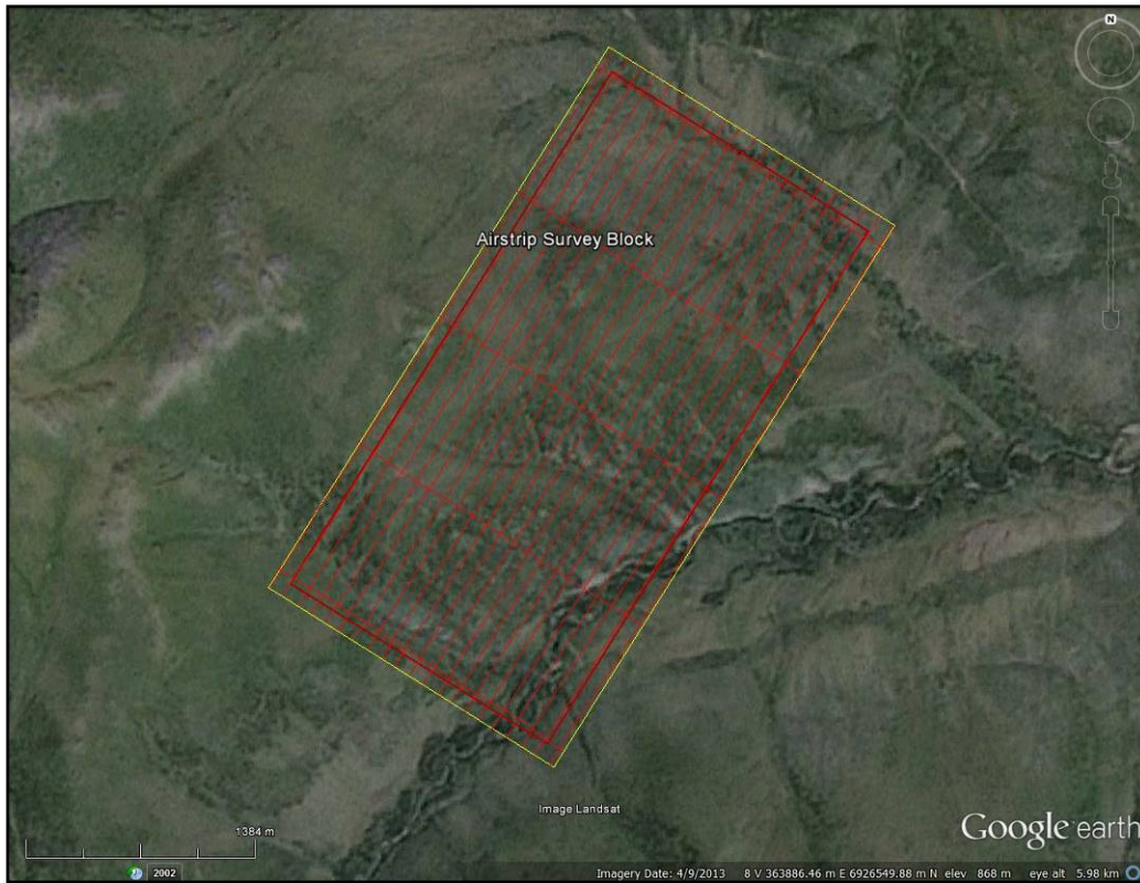
Figure 3: Plan View – Airstrip survey block with actual survey and tie lines displayed in red, the 100 m buffer zone outline in yellow, and the block boundary in brown.
