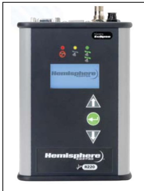
Figure 17: Hemisphere R220 GPS Receiver.
