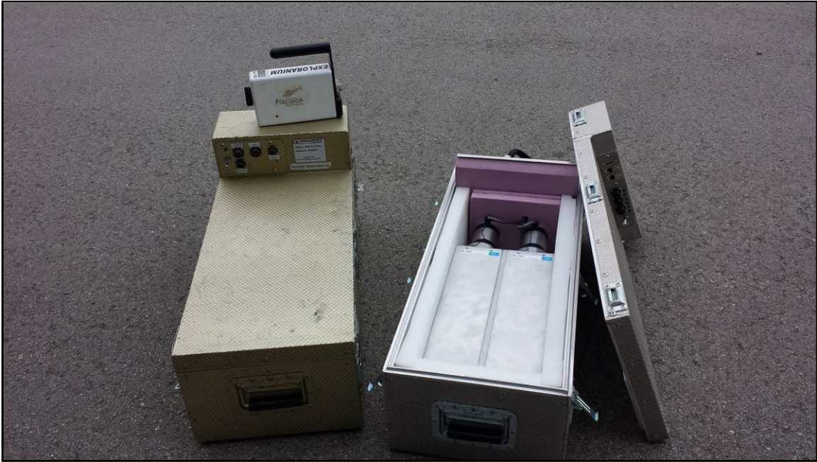
Figure 13: GRS-10 Thallium-activated Sodium Iodide spectrometer crystal pack.
