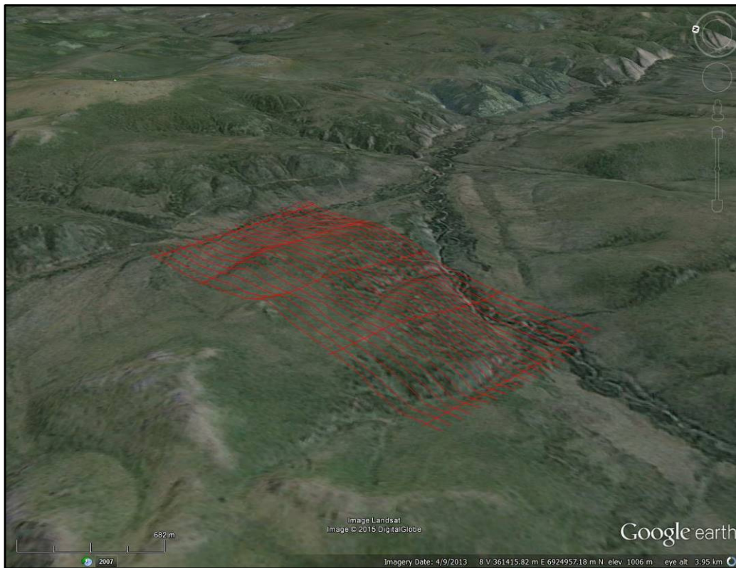
Figure 4: Terrain View – Airstrip survey block with actual survey and tie lines displayed in red.
