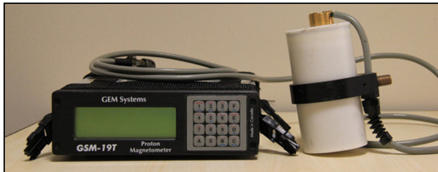
Figure 14: GEM GSM-19T proton precession magnetometer.
