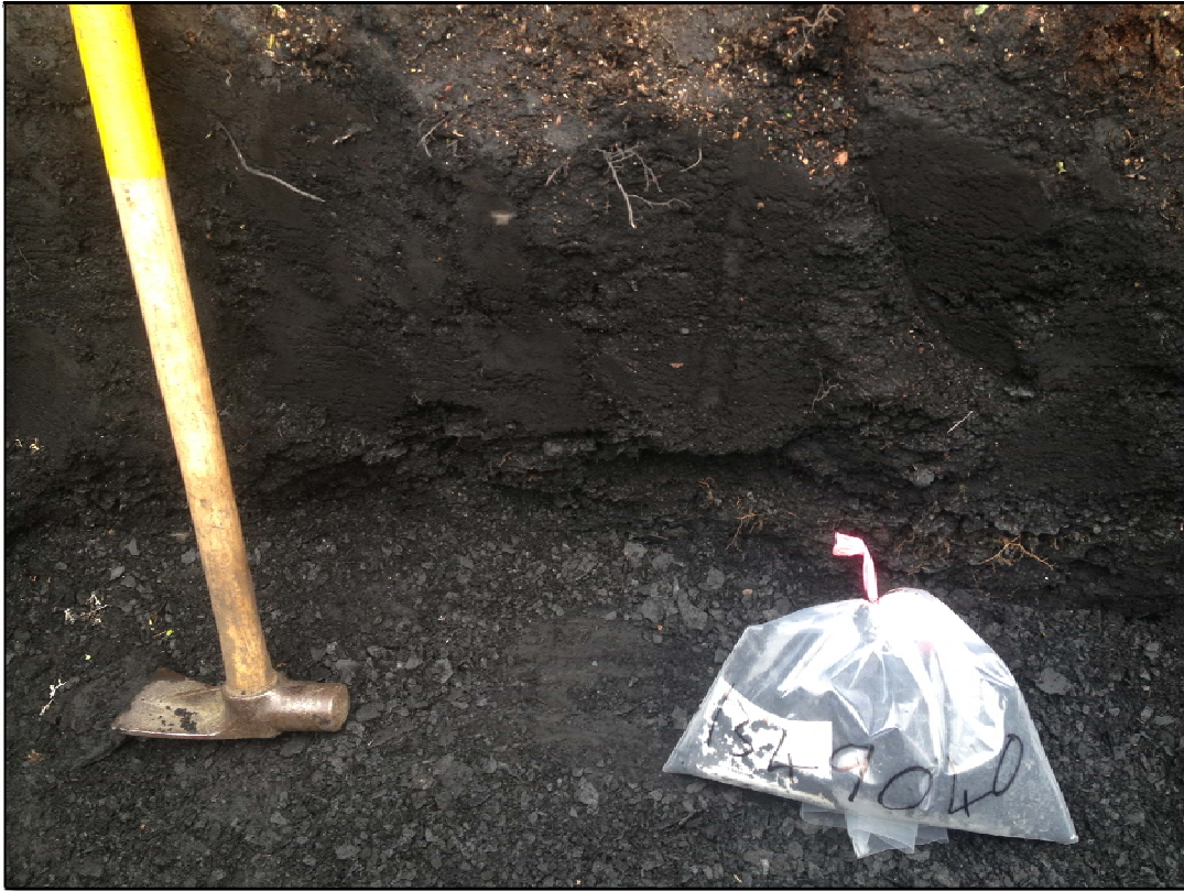
Trench 13-1.; rock sample 1349040 from trench floor black shale returned 63,000 ppb Ag, 445 ppm Cu, 1342 ppm Hg, 82.34 Mo, 19.71 ppm Sb and 1.41 ppm Tl.
