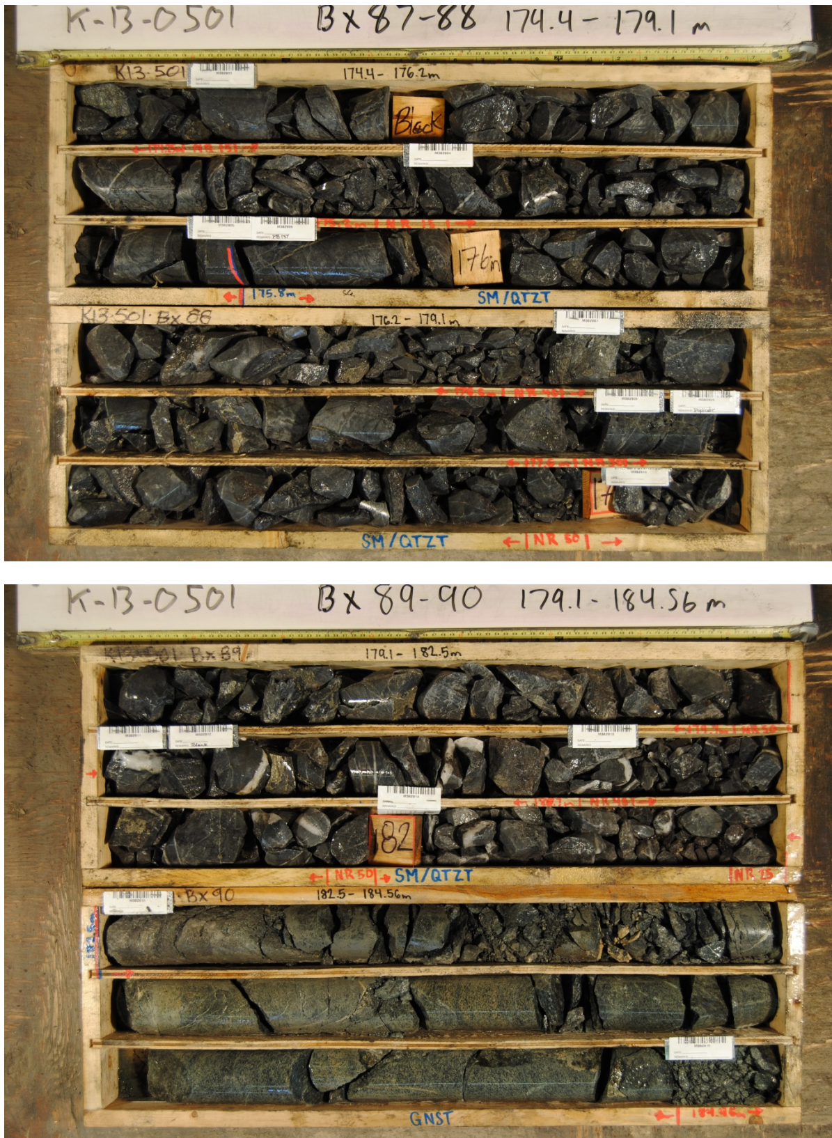
Figure 6. Core photos showing the main structure of the Bulldozer Vein fault (175.80 – 182.25m).
