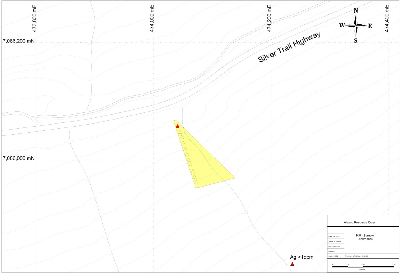
Figure 5. Highlighted symbol shows anomalous silver value from the 11 soil samples taken across the K 91 claim.
