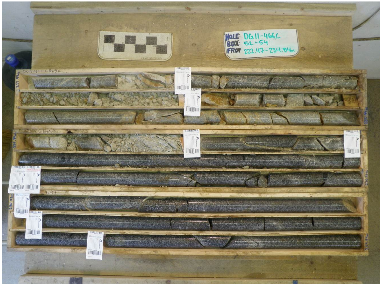
Figure 3 - Representative example of diamond drill core showing variable alteration
