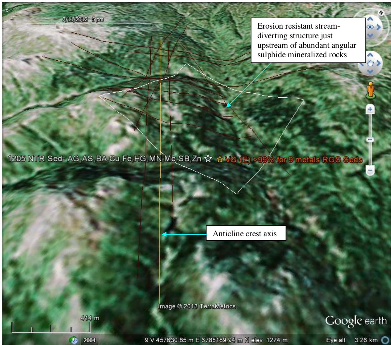
Map 7. Van Gogh (E) Area Recessional Features. The area has many linear recessive linements (faults?) (coloured brown) parallel to the stream and at the crest of the carbonate anticline (coloured yellow gold) which is to the west of the main stream. Other recessional features (faults?) intersect the carbonate anticline crest axis. BOLD assay highlights are 98-99 th percentile (ex. HG), normal are 90-95 th percentile (ex. Fe). View looking NNW.
