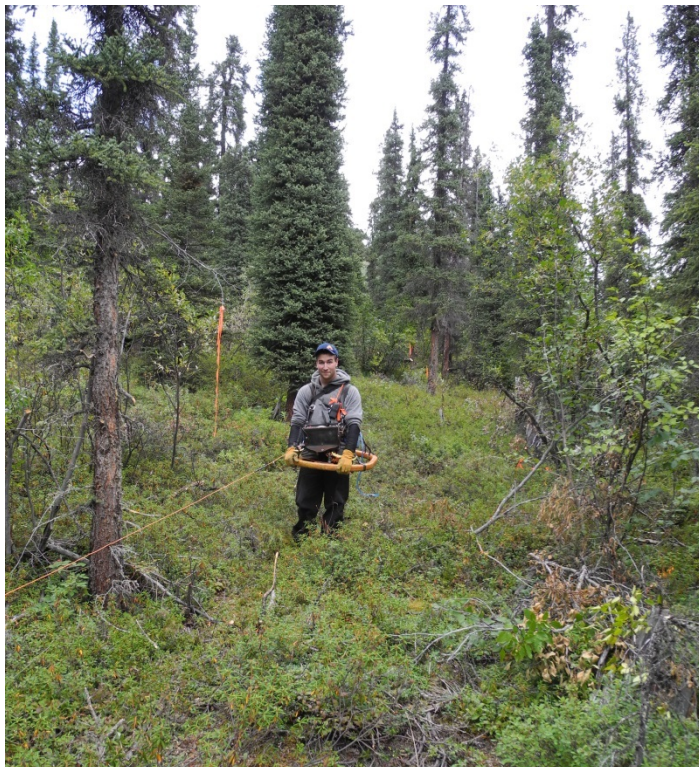
Figure 10: HLEM Survey. The field assistant with the receiving coil waits at a station while the reading is recorded.
