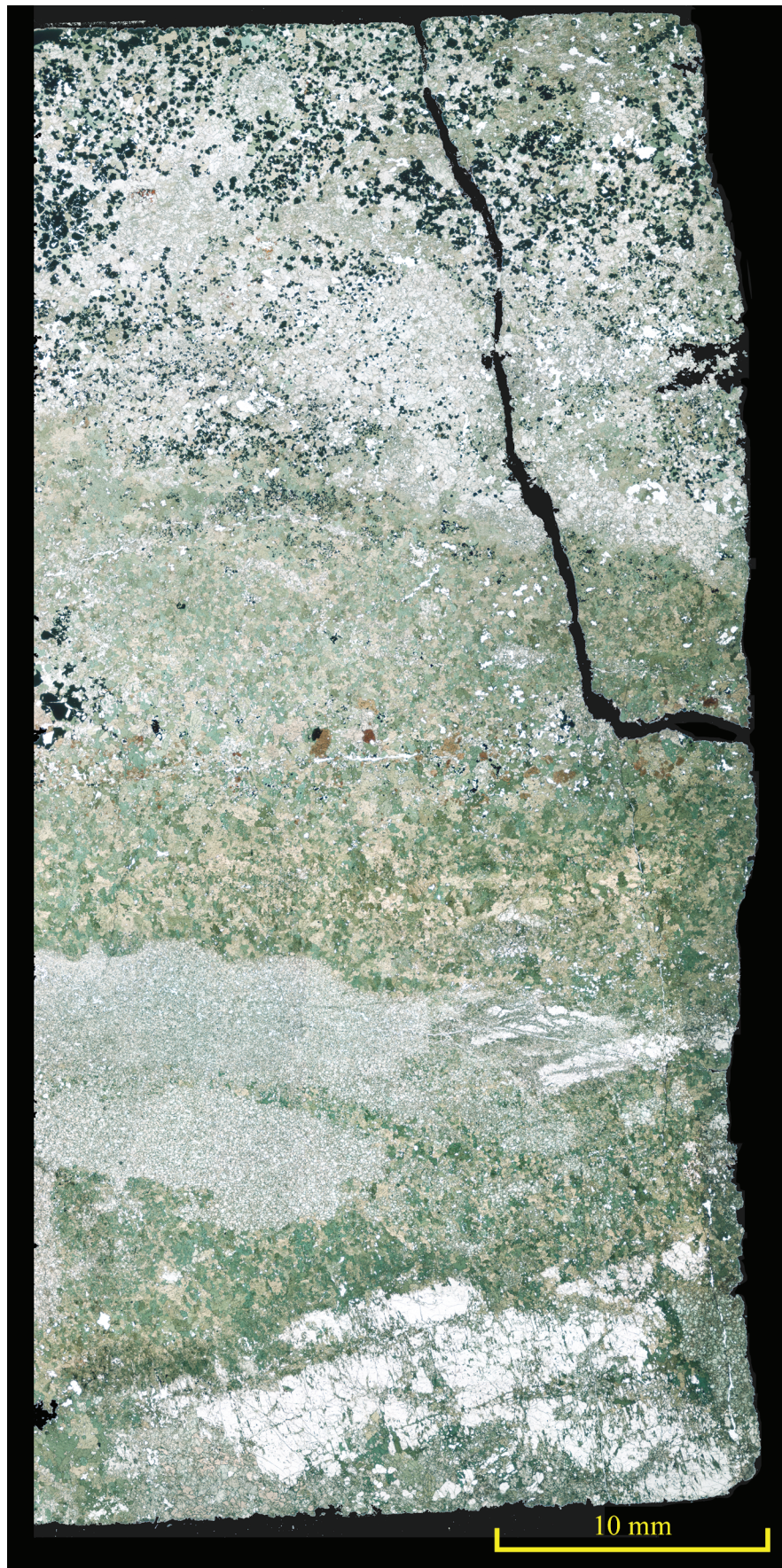
Figure 7. Thin section of specimen V8 under crossed polarisers. 'Stitched' mosaic of > 80 photomicrographs to show the complete length of the slide.
