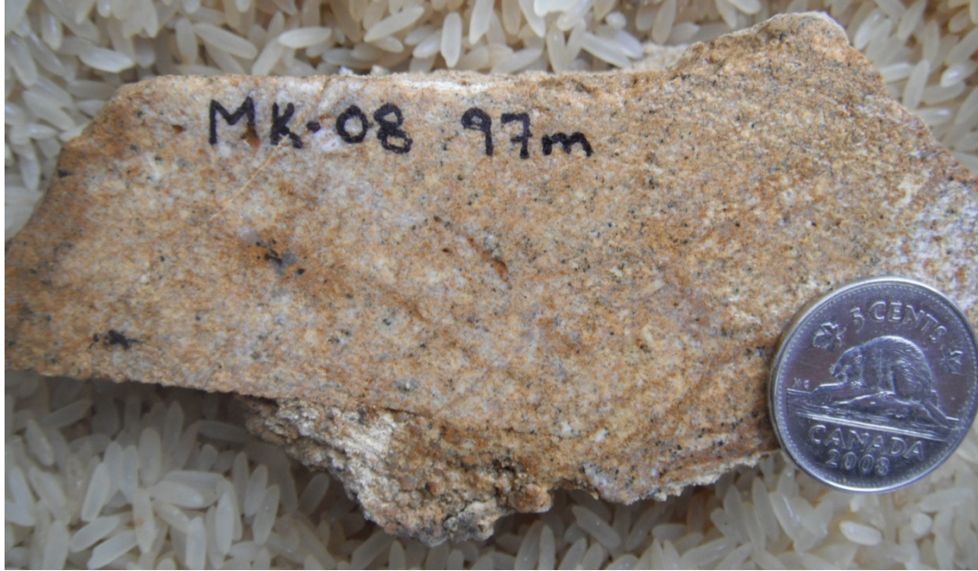
Figure 37: Hand sample of strongly altered rock from WGMK12TR08 at 97 m. Assay results for the channel sample from 95 – 100 m is 0.524 g/t Au.
