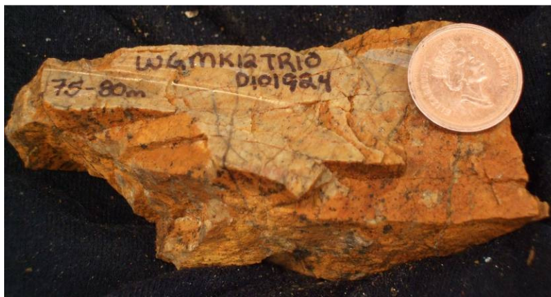
Figure 41: Hand sample from WGMK12TR10 at 75 – 80 m. Rock is intensely altered felsic gneiss with thin grey quartz veinlets and stringers. The 5 m channel sample over this interval contains 0.138 g/t Au.
