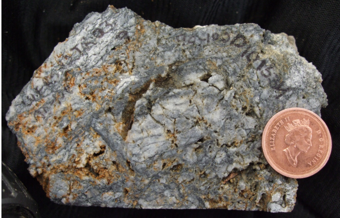
Figure 45: Hand sample from trench WGRS12TR03 at 95 m. Rock is brecciated banded quartzite. Gold grades within this breccia are 1.72 g/t Au, over 10 m, from 90 – 100 m. The gold is also associated with thin quartz-carbonate veins with cubic pyrite.
