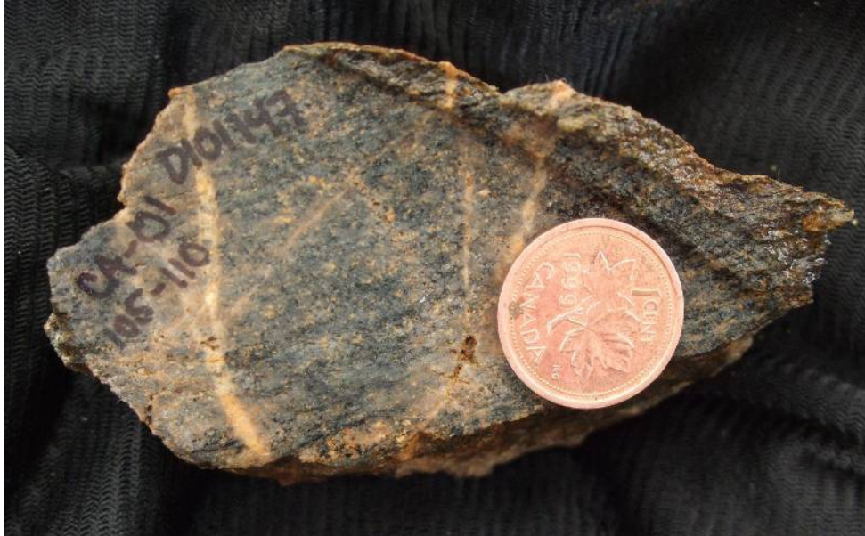
Figure 21: Representative hand sample from 105 – 110 m in WGCA12TR01, showing thin quartz veinlets. The interval from 100 – 115 m contains 0.114 g/t Au over 10 m. A spot sample collected at 104 m contains 1.64 g/t Au.
