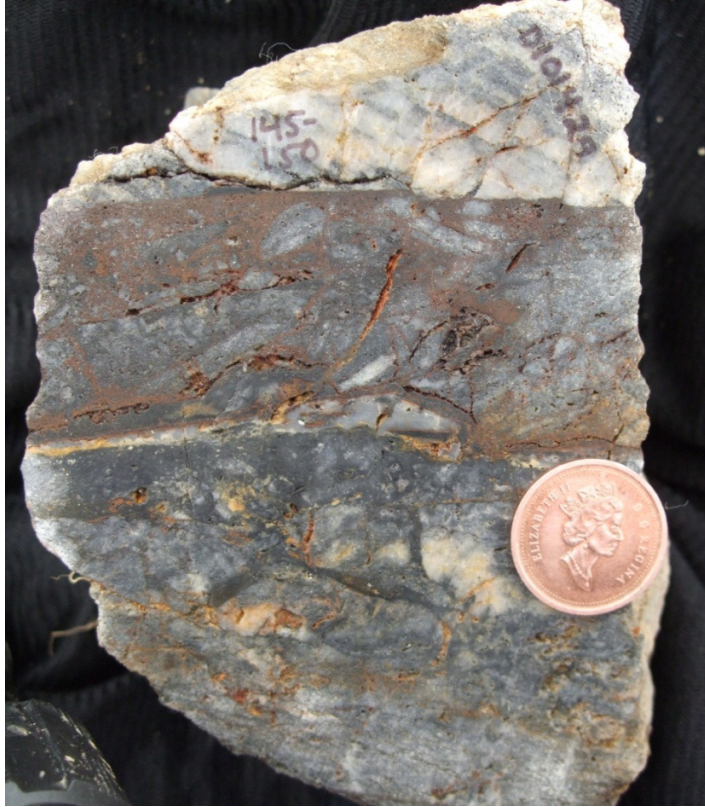
Figure 50: Hand sample from WGUR12TR01 at 145 – 150 m. Rock is brecciated banded quartzite. The gold assay result from the 5 m channel sample at 145 – 150 m is 0.193 g/t Au. This is within a larger interval from 130 – 150 m, with an average of 0.569 g/t Au.
