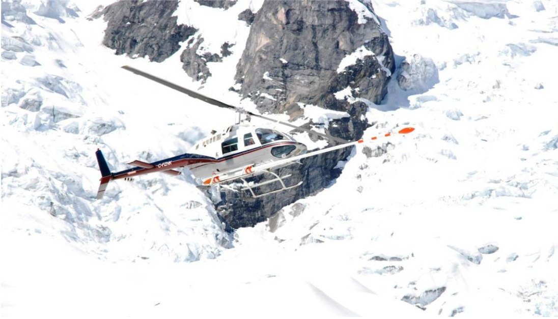
Figure 12: Bell 206 Jet Ranger helicopter equipped with mag stinger for magnetic data acquisition.
