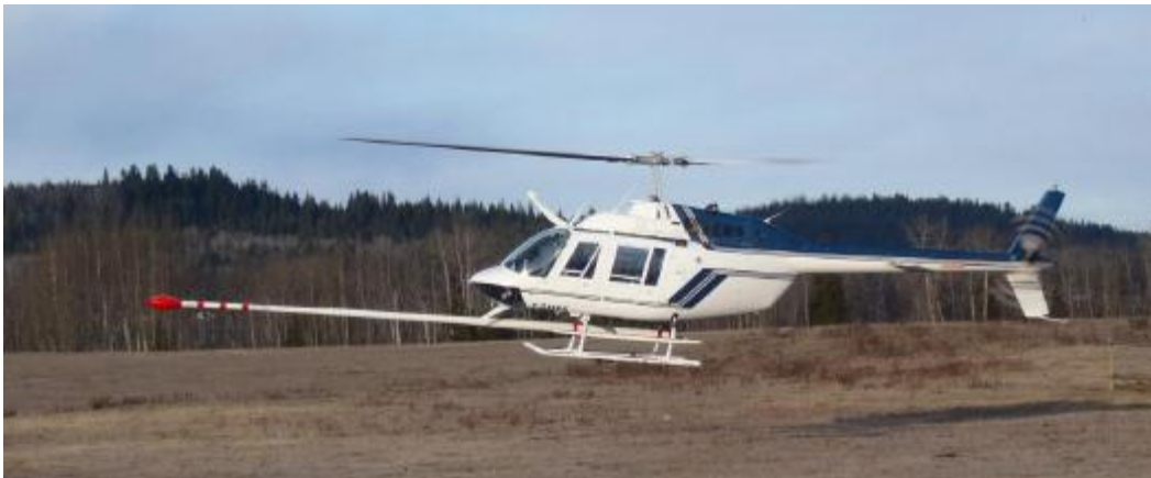
Photo 3: Northern Air Support Bell 206 B3 helicopter with magnetometer mounted in a fixed stinger assembly used in survey.
