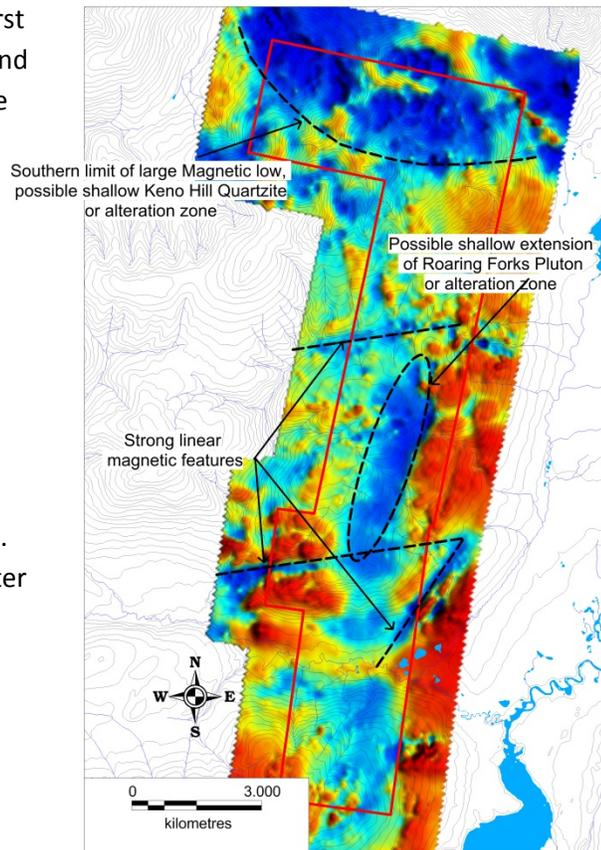
**Figure 7** Total magnetic intensity map from survey Block A
