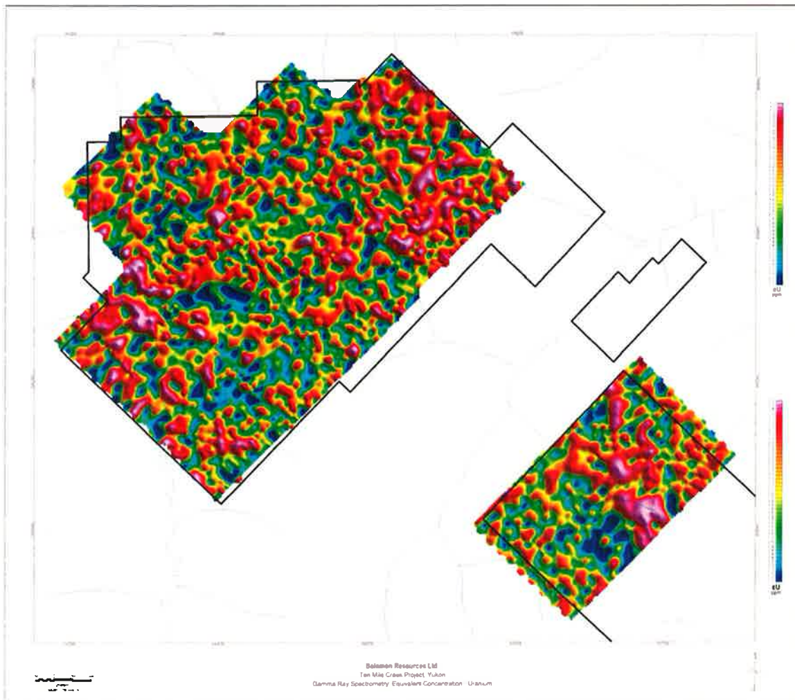
Figure 9. Gamma-ray spectrometry: Equivalent Concentration – Uranium
