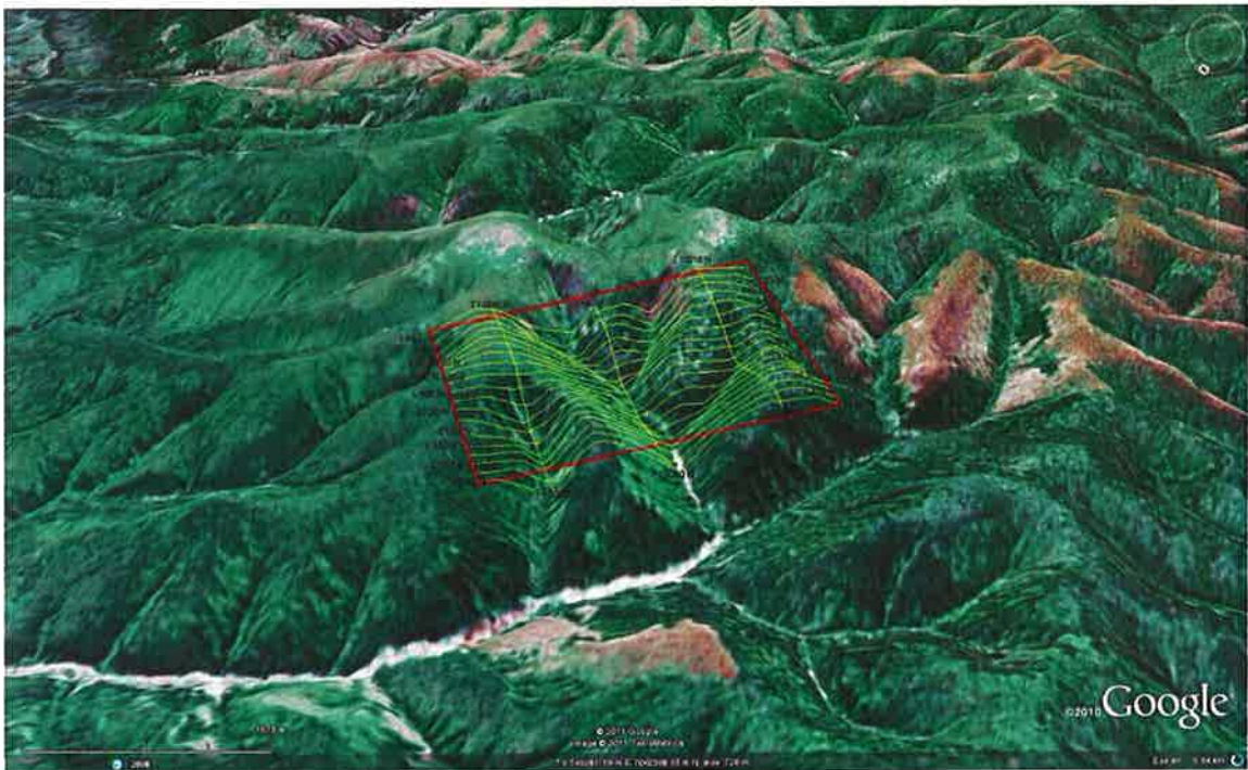
Figure 5: Block B with survey and tie lines outlined in yellow and the boundary in red in terrain view.
