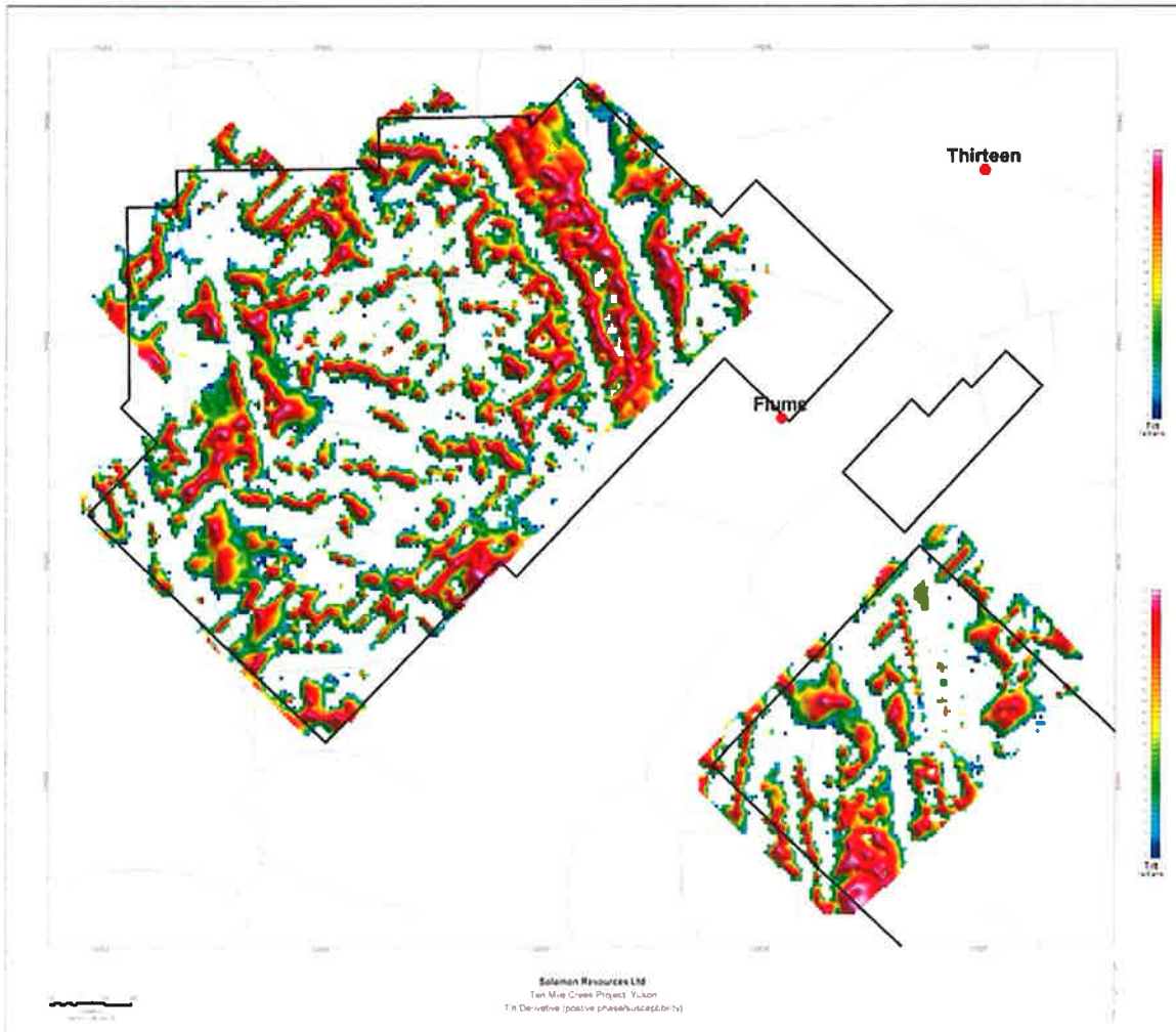
Figure 16. Tilt derivative clipped to positive phase only
