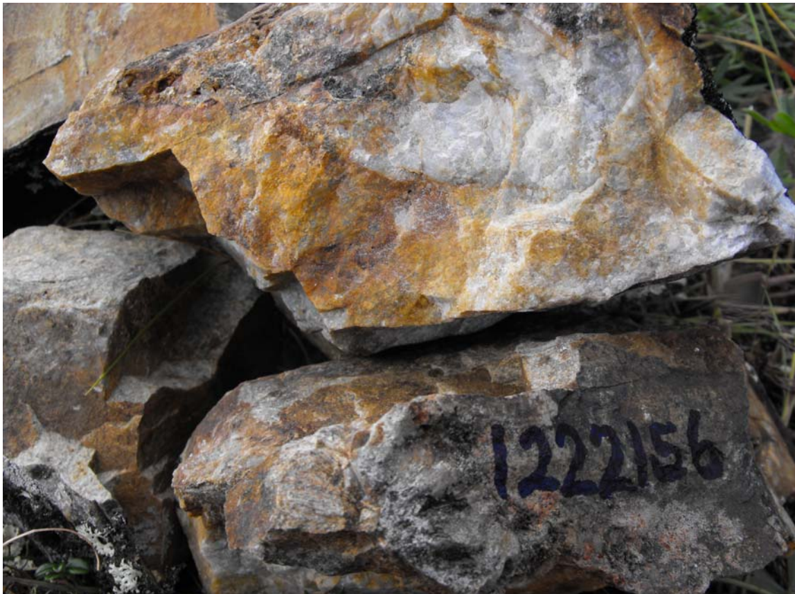
Photo 2: Sample 1222156 displays typical appearance of the metasediment hosted quartz veining on the Property.
