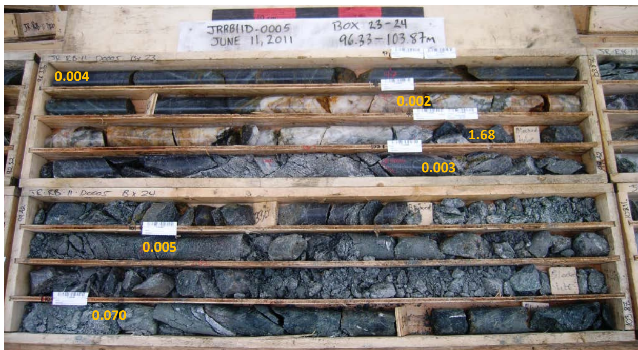
Figure 6: Gold assay results (g/t Au) from hole JRRB11D0005. A high-grade quartz vein occurs with 1.68 g/t Au from 98 – 99 m. Pyrite, chalcopyrite, occur within the vein, along with trace molybdenite and bornite.
