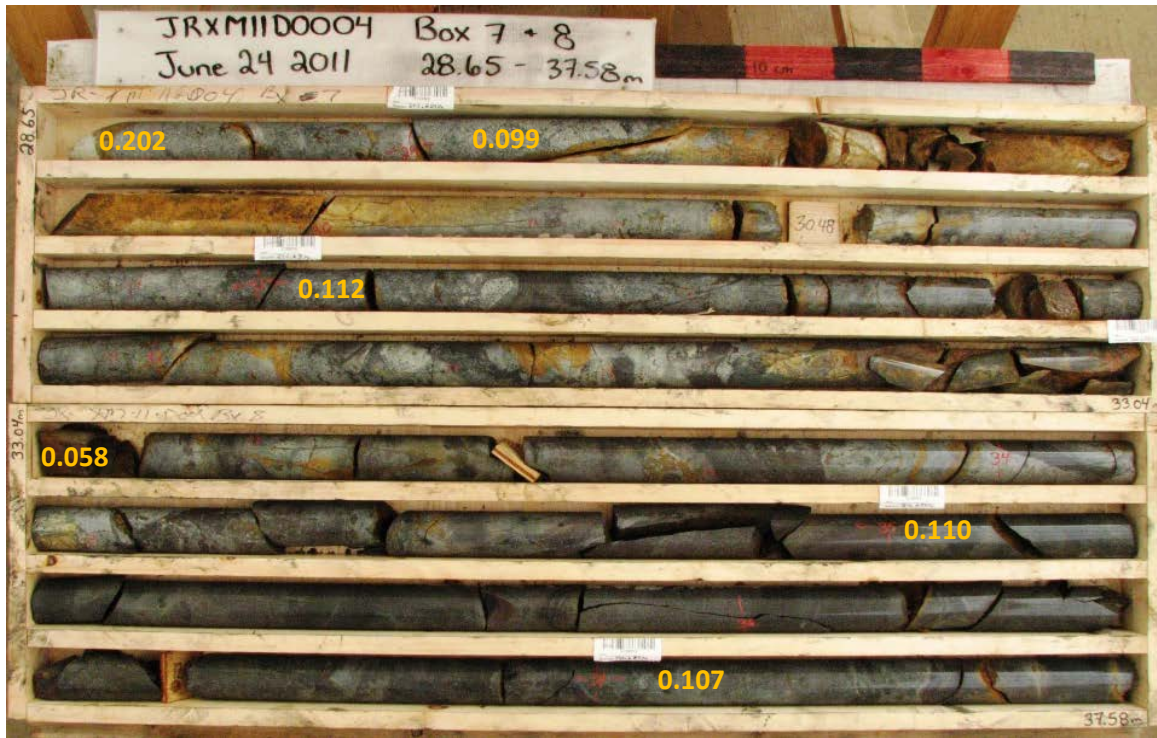
Figure 10: Gold assay results from JRXM11D0004. Low gold occurs over a 58 m interval (average 0.11 g/t Au). This photo shows the transition from underlying Carmacks lapilli tuff to hornblende-feldspar porphyry.
