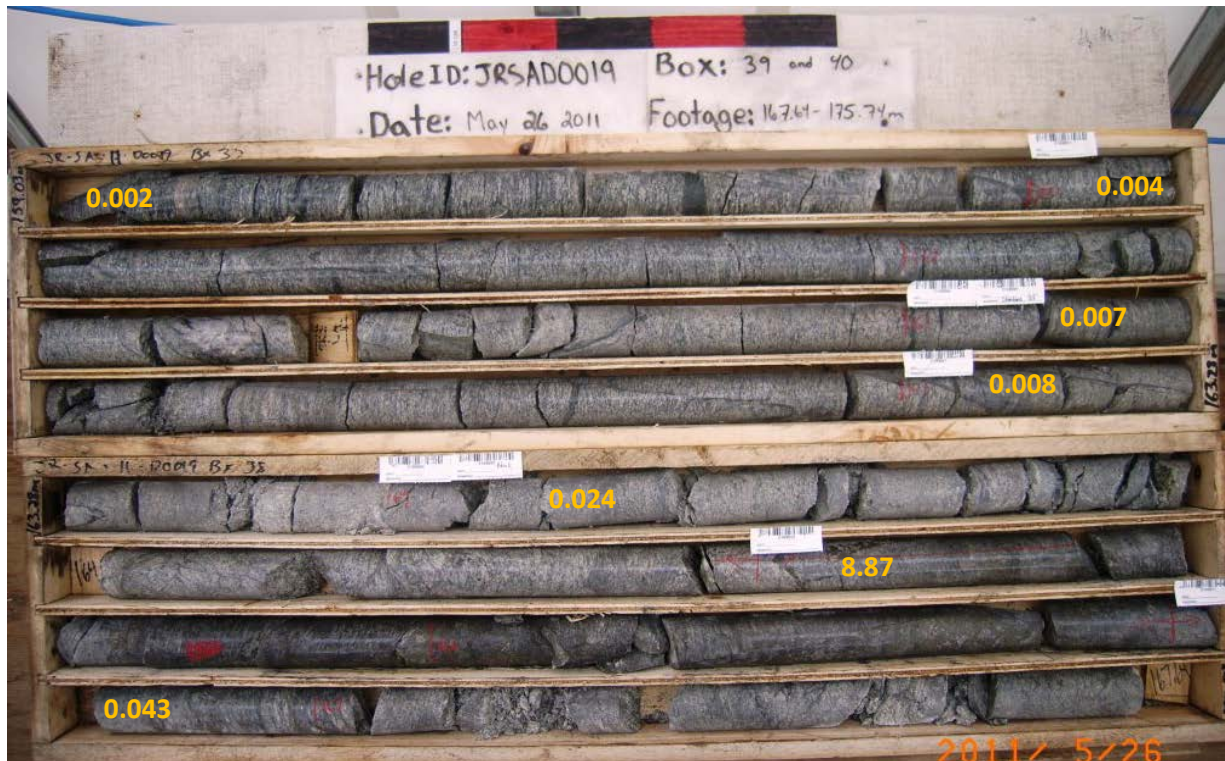
Figure 8: Gold assay values (g/t Au) from hole JRSA11D0019, 159.03 – 167.64 m. A high-grade quartz-pyrite vein occurs from 165.2 – 166.75 m, with 8.87 g/t Au. This vein contains ~50% pyrite, and is hosted within BQFG.
