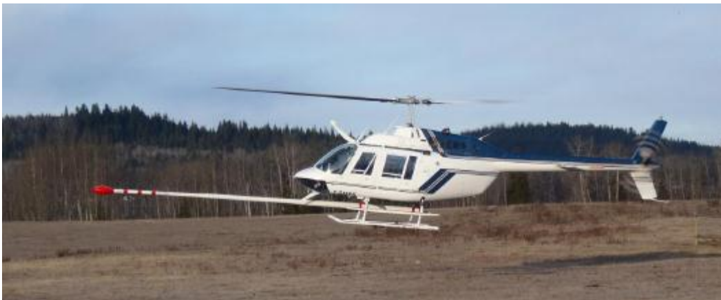
Photo-Plate 3: Northern Air Support Bell 206 B3 helicopter with magnetometer mounted in a fixed stinger assembly used in survey.
