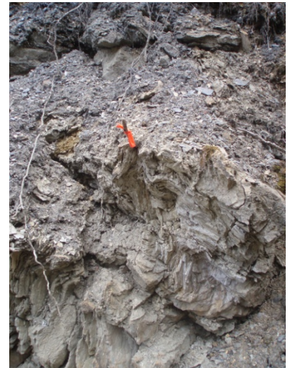
Figure 8. Graphitic argillite above phyllite (Stn RC07)
