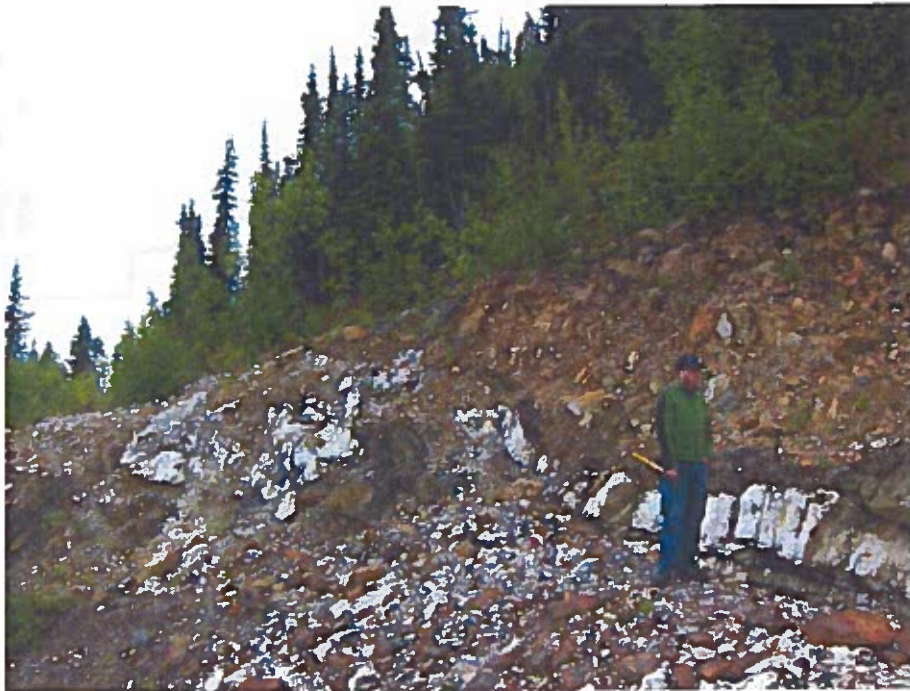
Plate 3 - TOG Massive quartz vein bounded by graphitic sheared ultramafics with listwanite alteration
