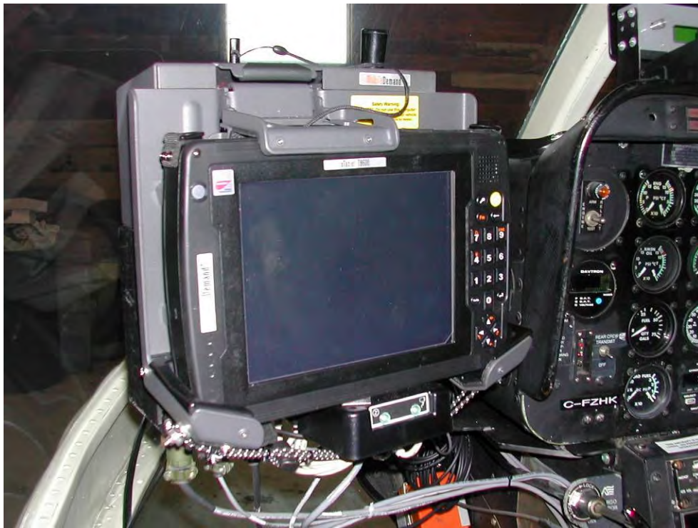
Figure 6: AGIS installed in the Bell 206.
