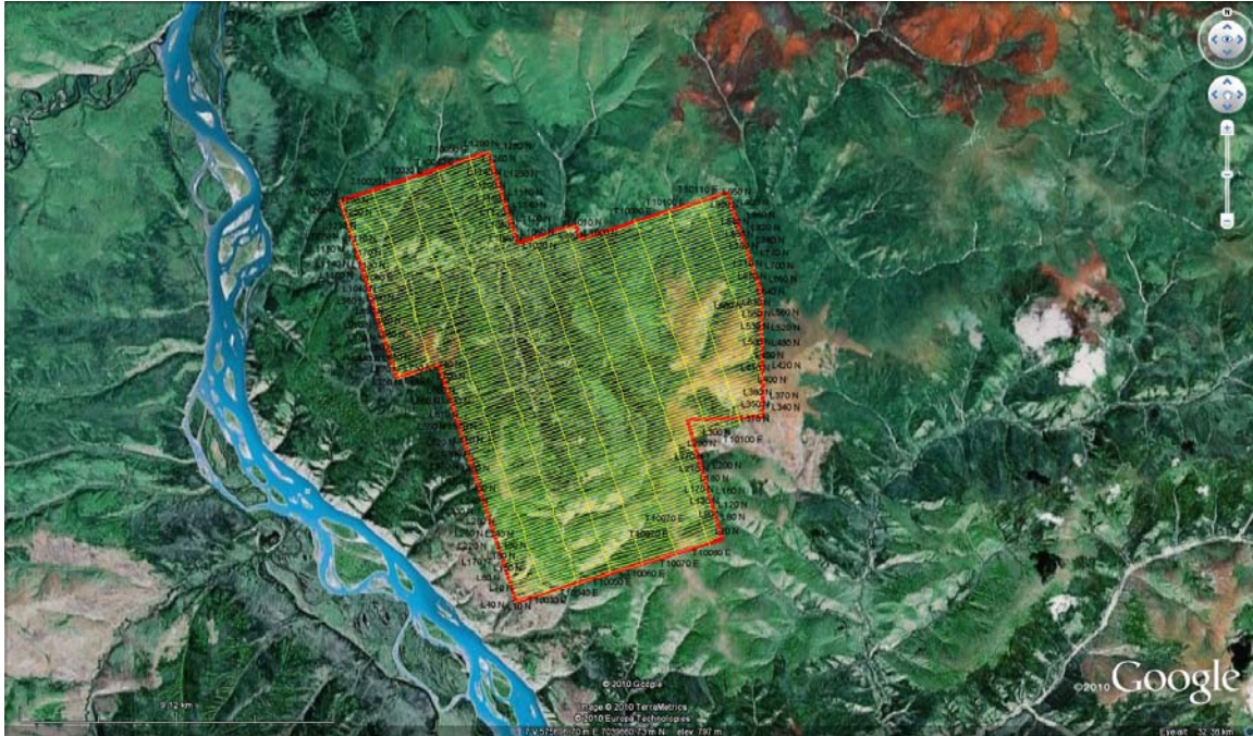
Figure 2: Survey and tie lines outlined in yellow and the boundary in red.
