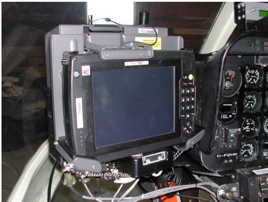
Figure 6: AGIS installed in the Bell 206.
