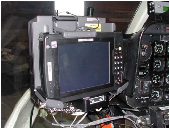
Figure 4: AGIS installed in the Bell 206.
