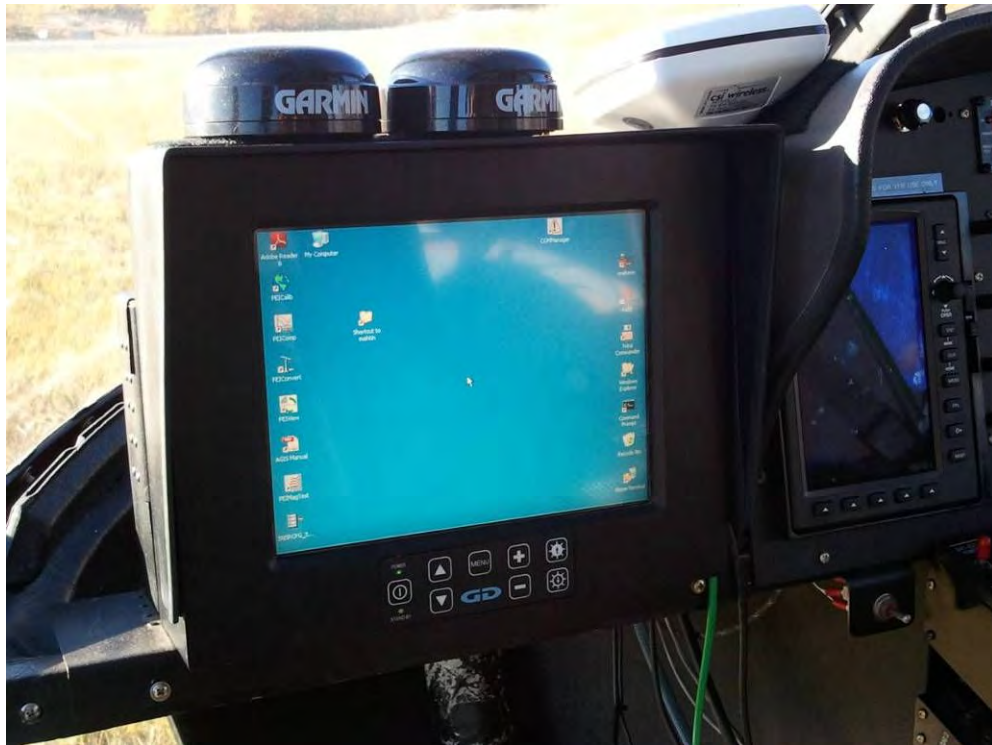
Figure 6: AGIS installed in the Bell 206 Long Ranger
