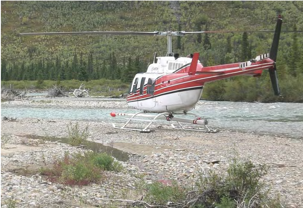
Figure 5: Bell 206 Long Ranger equipped with mag stinger for magnetic data acquisition
