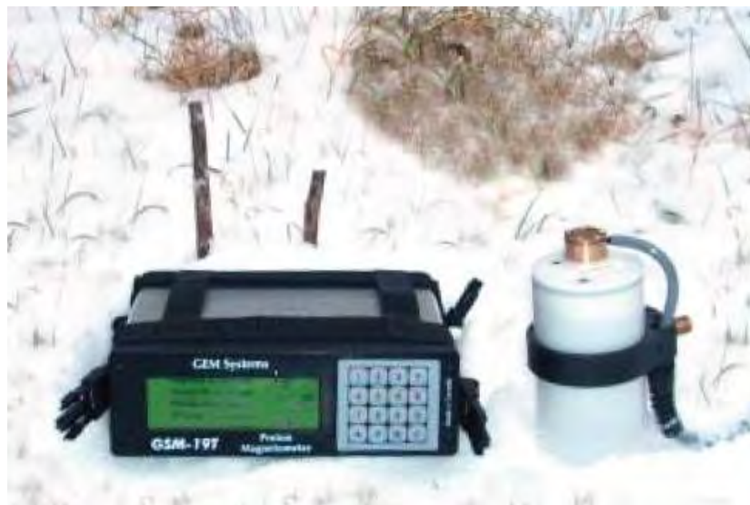
Figure 9: GEM GSM-19T proton precession magnetometer.
