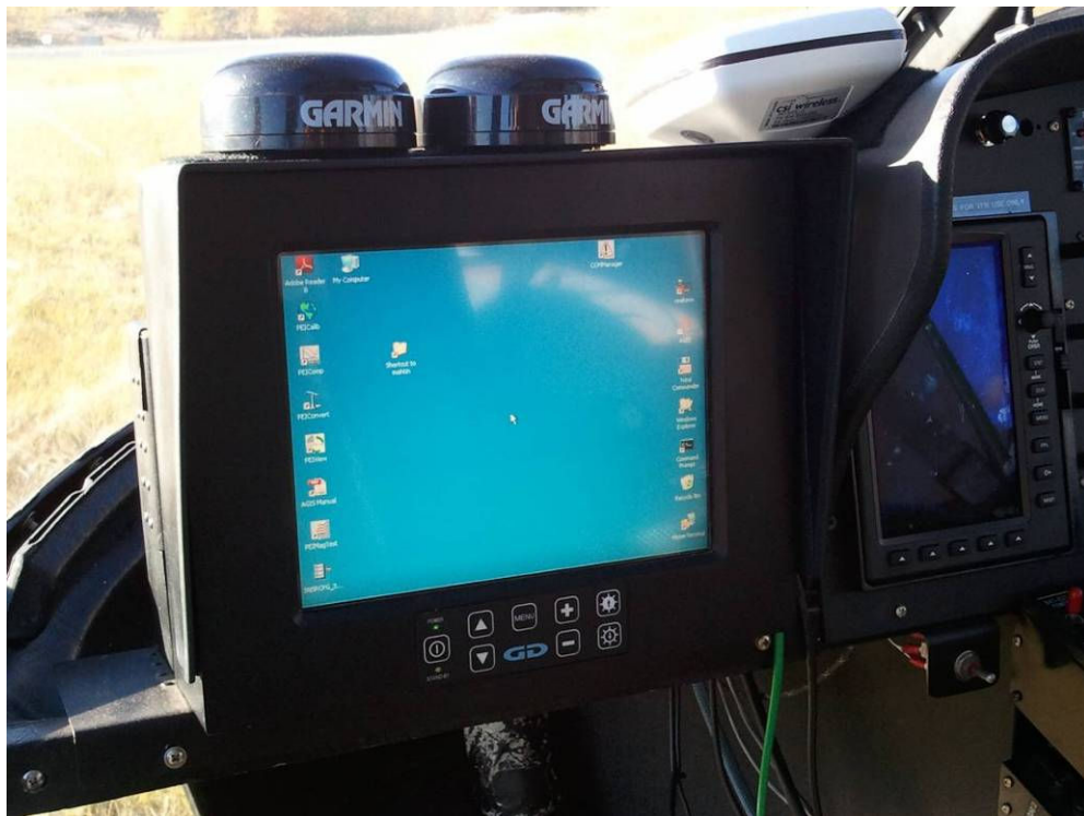
Figure 6: AGIS installed in the Bell 206 Long Ranger
