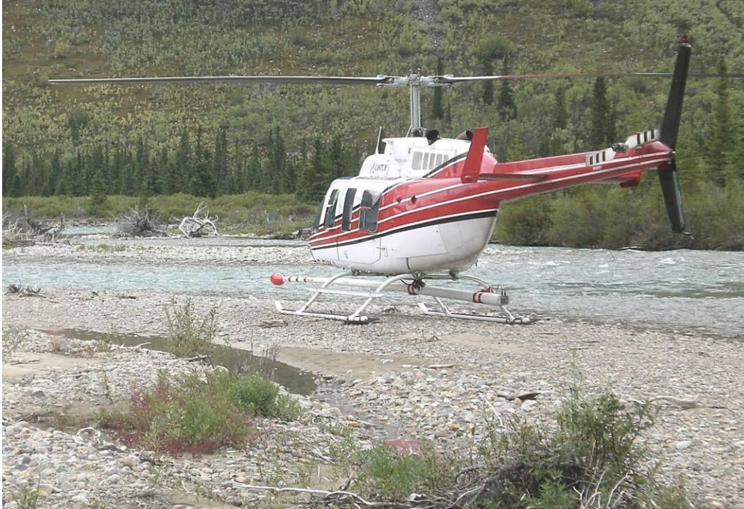
Figure 5: Bell 206 Long Ranger equipped with mag stinger for magnetic data acquisition
