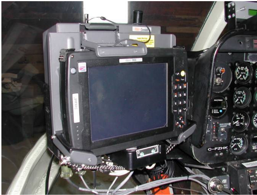
Figure 5: AGIS installed in the Bell 206.
