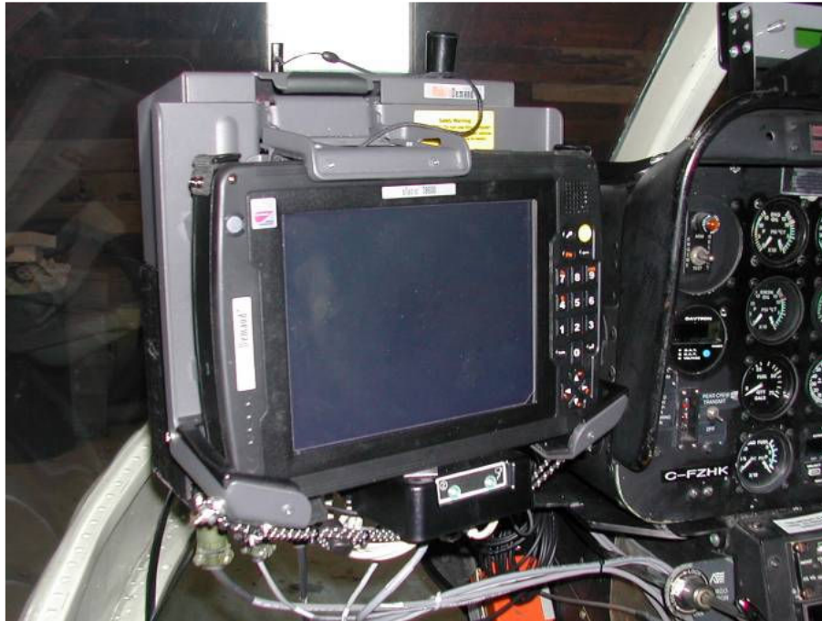
Figure 5: AGIS installed in the Bell 206.
