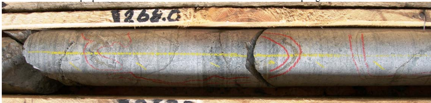
Figure 4: This photo shows a cut-line perfectly bisecting the veins. Notice the dashed yellow lines pointing to the end (left) of the box, this will aid the core-splitters when cutting and orienting the core.
