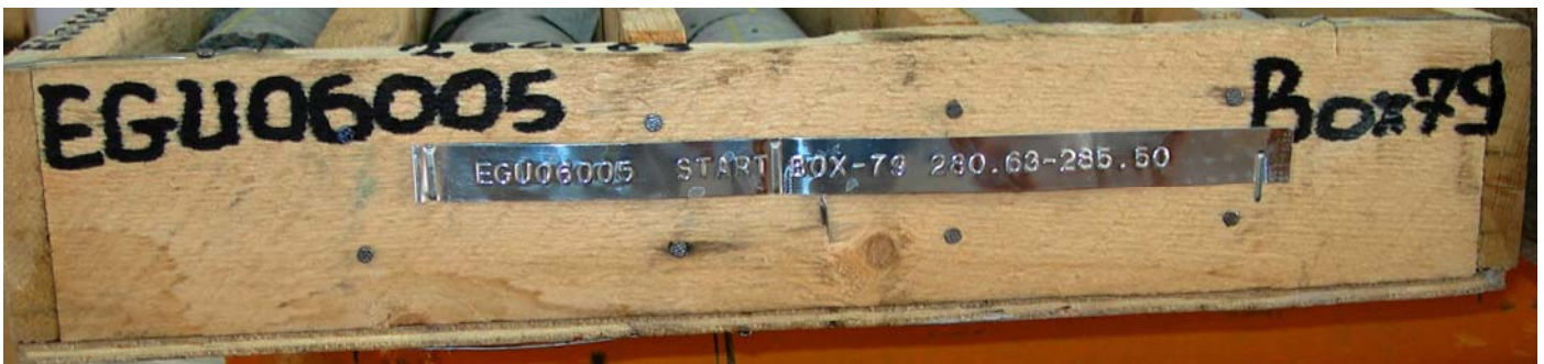
Figure 1b: Frontal view of the box with a clearly labeled aluminum tag reading the hole name, box number, and depth of core within the box.
