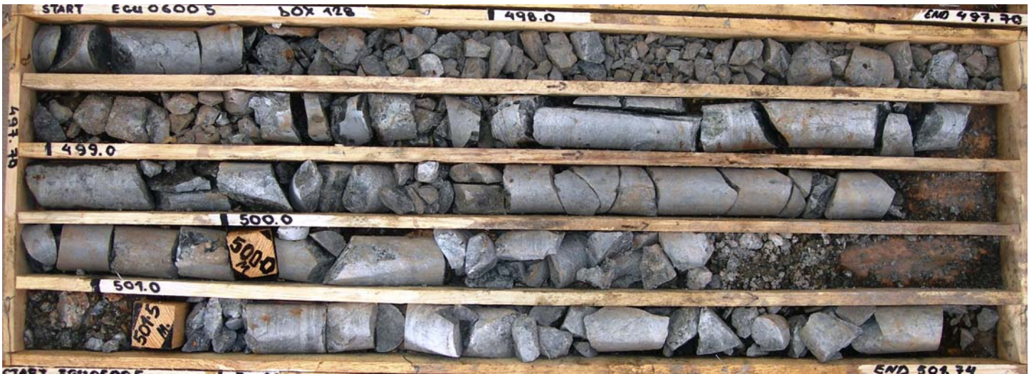
Figure 1a: Top view of a core box showing the correct layout and markings. The box is clearly labeled with the title, box number, start, end, and whole meter markings. These, along with the run-blocks, are easy to read.
