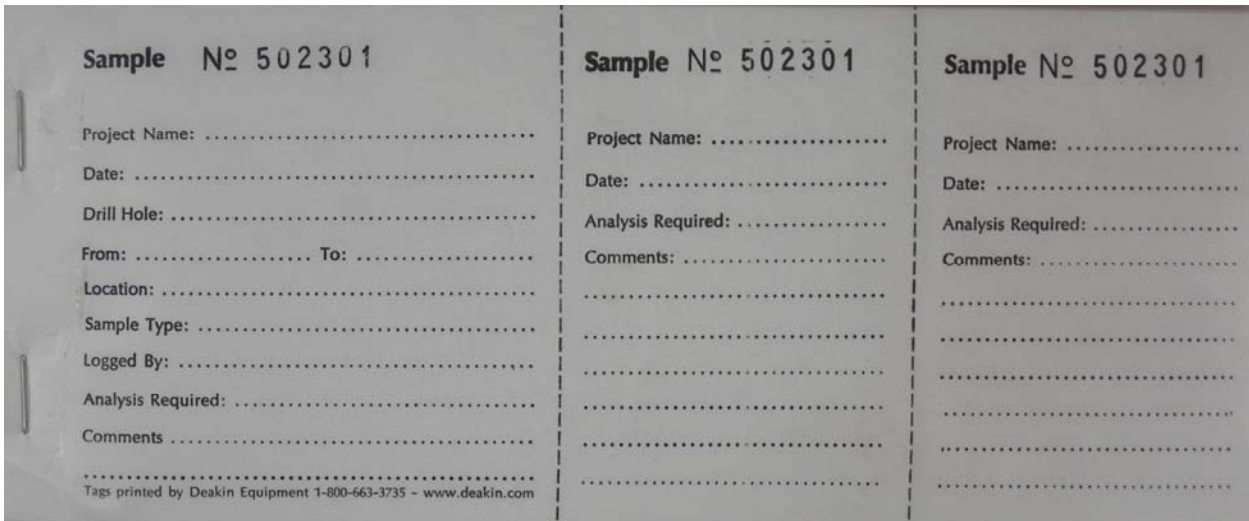
Figure 3: Typical assay book. The left ticket is filled out and saved, the middle ticket is stapled to the box, and the right ticket is sent with the sample.
