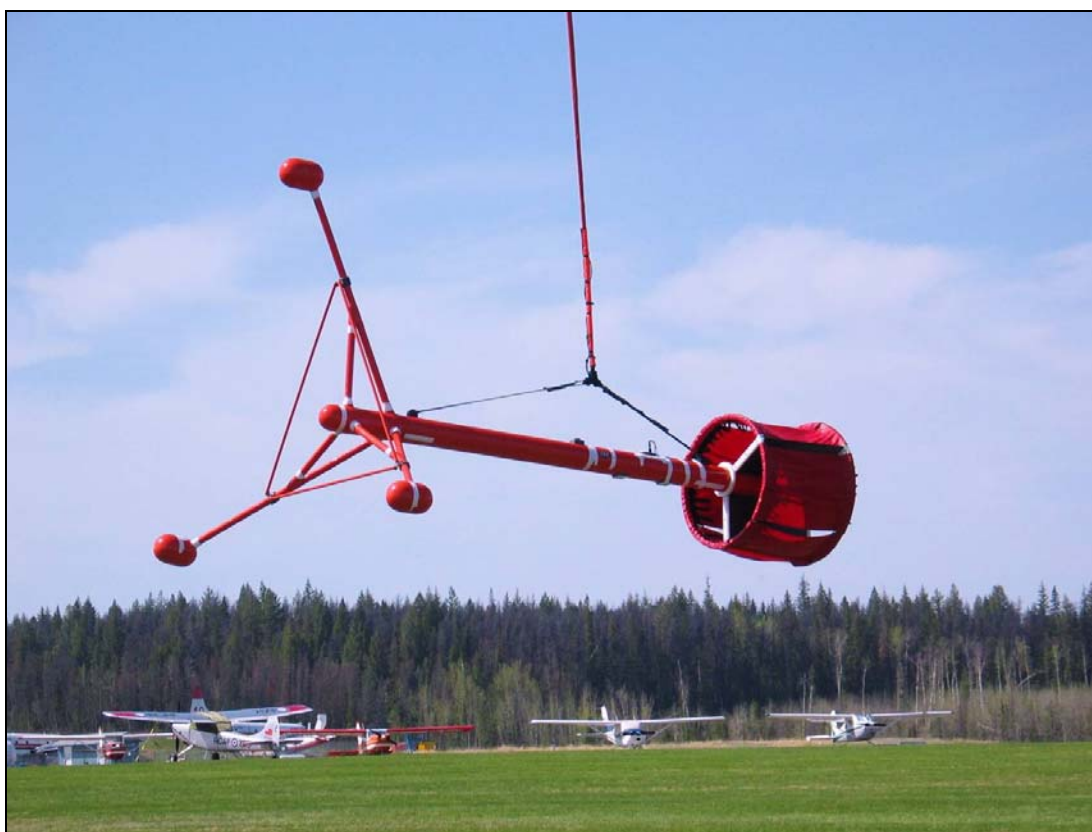
Figure 5 - The CMG tri-axial magnetic gradiometer.
