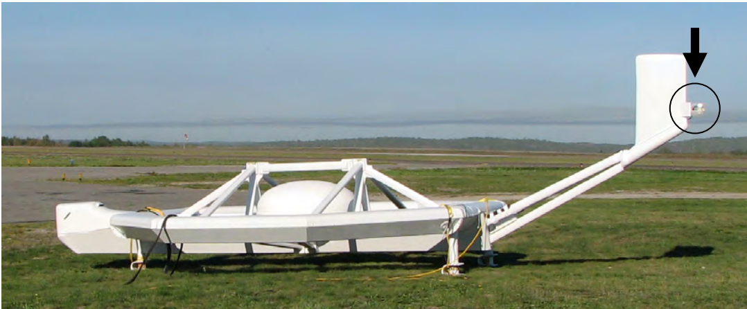
Figure 3. AeroTEM II EM bird. Arrow indicates the location of the second caesium magnetometer sensor.
