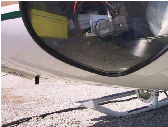
Figure 7. Digital video camera typical mounting location.
