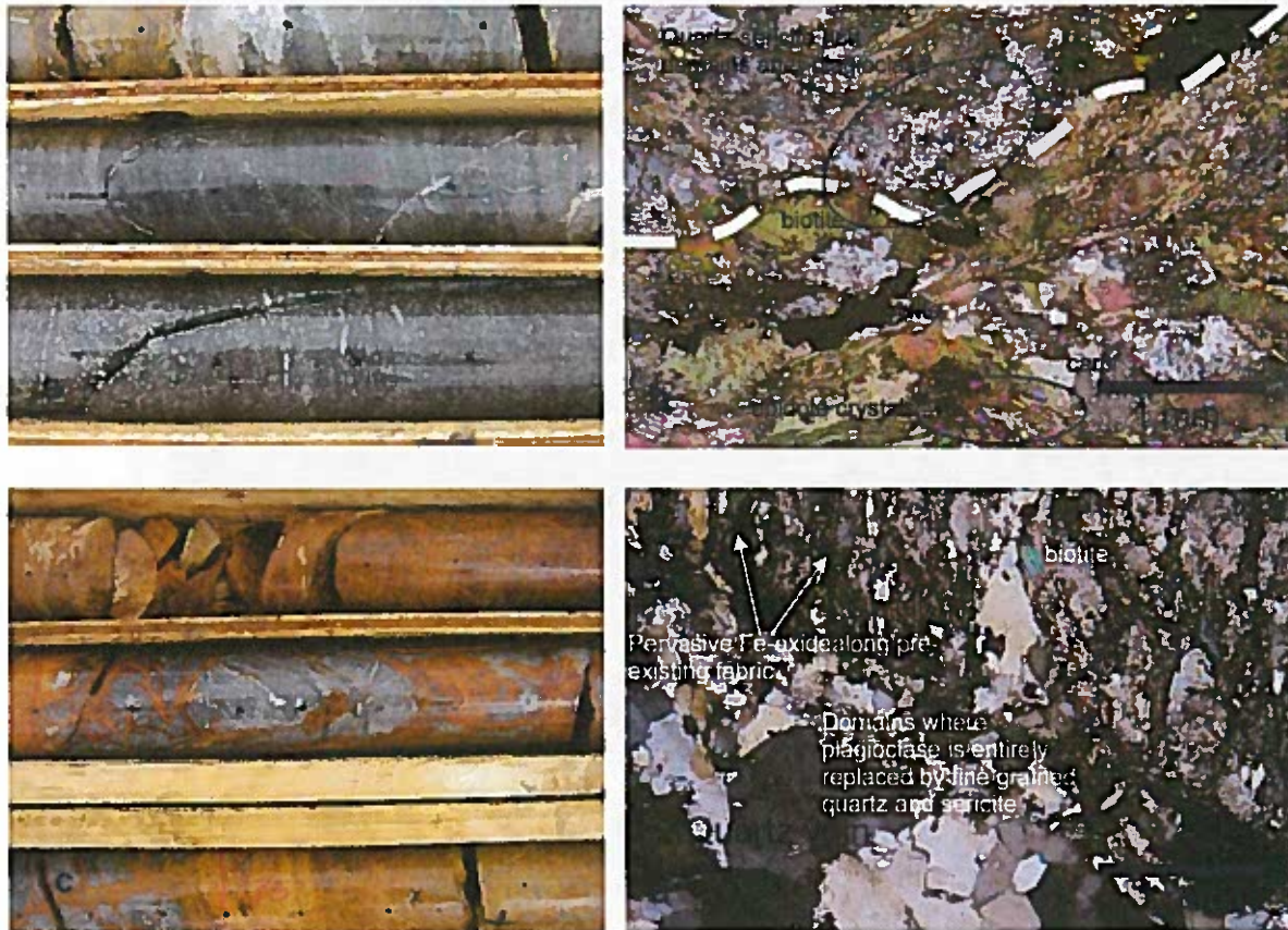
Figure 13. Latte. a. Quartz biotite schist, the dominant lithology at Latte. b. Photomicrograph of quartz biotite schist (x-nicols). Note primary pyrite along biotite ribbons. Secondary phases consist of plagioclase, epidote, carbonate and chlorite. Dashed white line shows fabric orientation. c. Mineralized biotite schist. Note the variable intensity of veining to the point of total replacement. d. Photomicrograph of mineralized quartz biotite schist (sample grade = 3.2 g/t Au). Plagioclase replaced by fine-med grained mica (sericite) quartz and secondary carbonate. 30 to 40% of rock is quartz. Oxidized pyrite is pervasive along pre-existing fabric.
