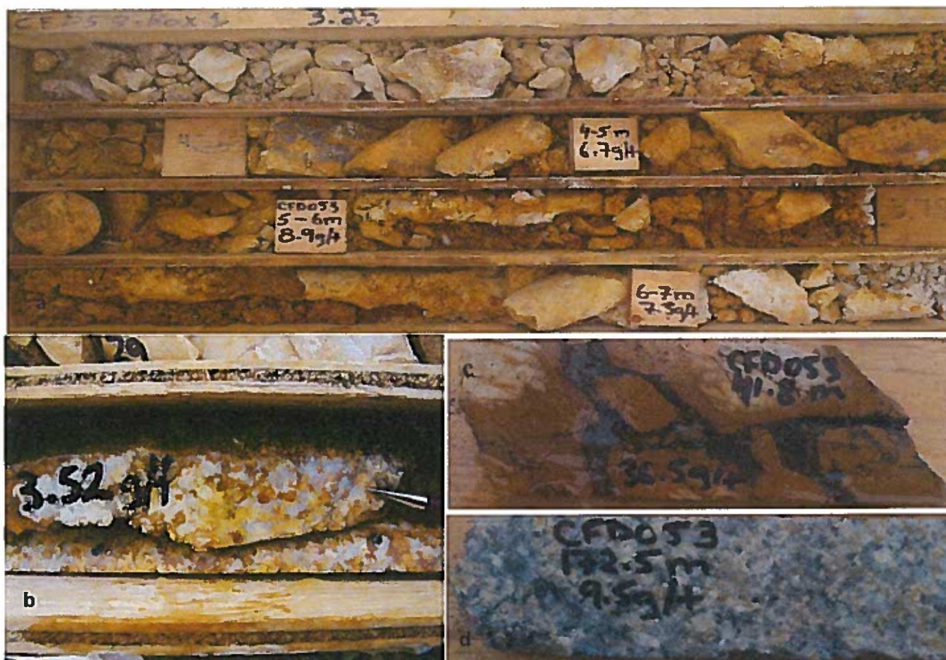
Figure 19. Kona Mineralization styles. a. Clay / limonite alteration of granite. Dacite dyke also occurs across the interval. b. Granite; clay and limonite altered; mottled silica and local oxidized pyrite cubes c. Clay / limonite altered dacite dyke; Silicified and brecciated. d. Albitized / sericitized granite; Mineralization controlled by sulphide (steel grey mineral) replacement of amphibole.
