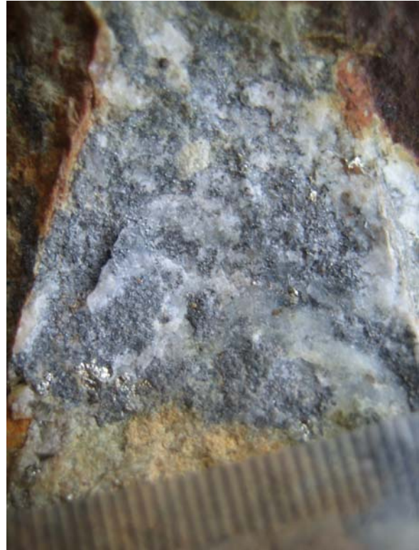
Sample RS-68, Fine-grained aspy masses with late py in qz-cb vein
