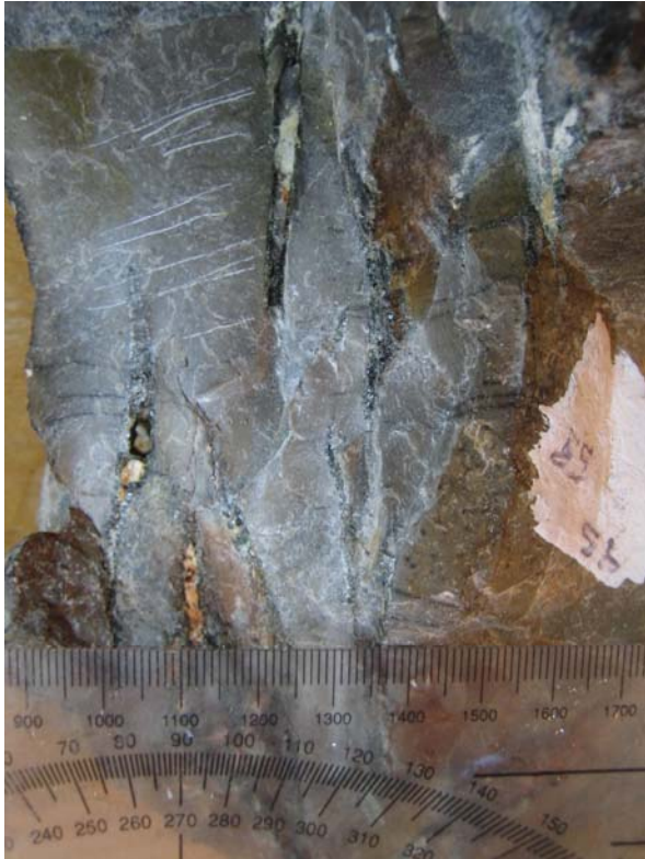
Sample RS -53, Sericite phyllite with orthogonal dilatant vein sets with aspy
