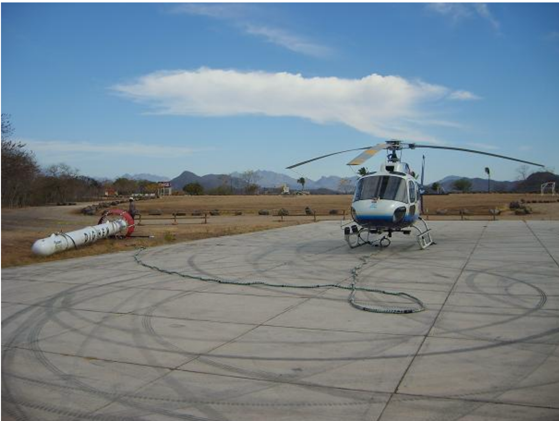
Figure 1: Fugro Airborne Surveys DIGHEM EM bird with AS350-B3
