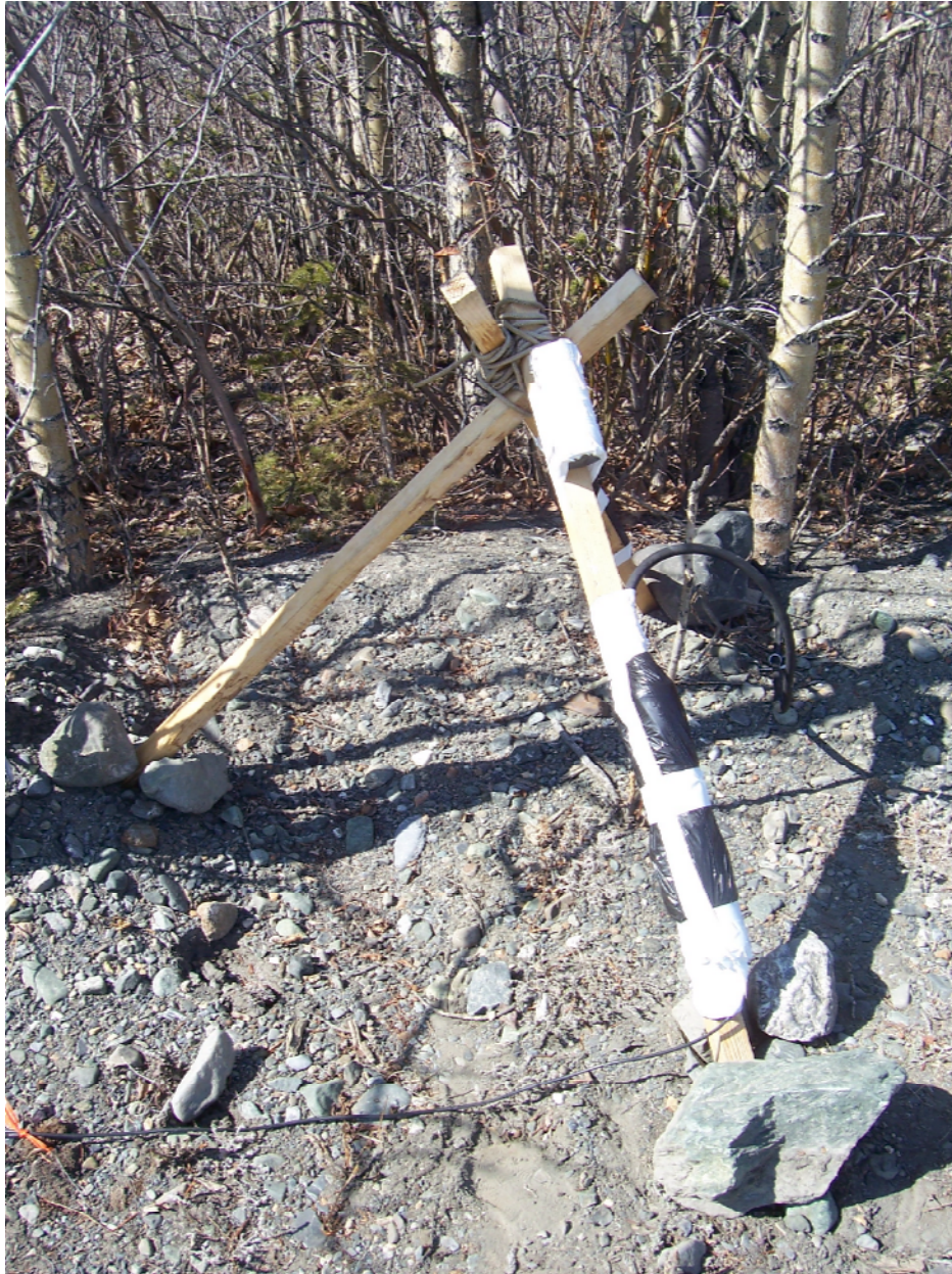
Figure 3 Primary Magnetic Base Station
