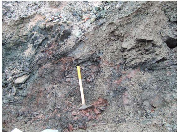
Photo 2. Potassically altered and hematized sediments in the DEER Showing shear zone.
