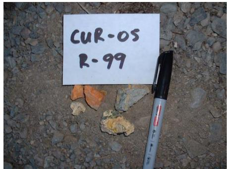
Photo 7. Hi-grade uranium (carnotite(?)) mineralization from Deer Showing (54% wt  $U_30_8$ )
