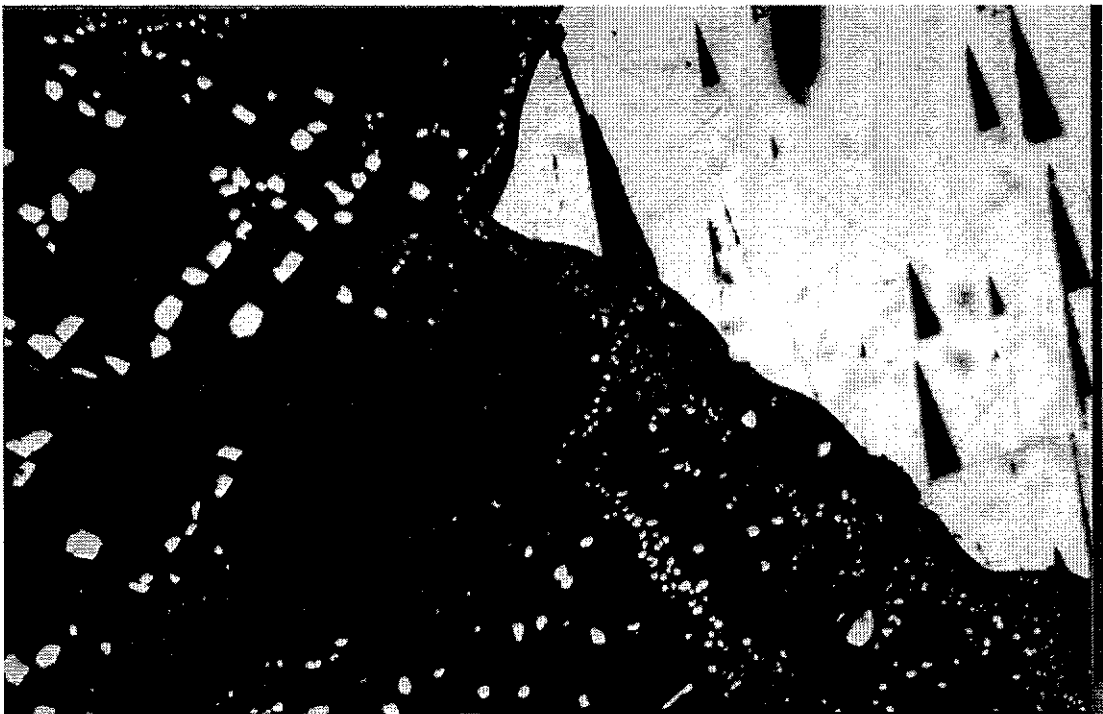
Figure 9. TBMB trench 5b. Pyrite and galena in sphalerite. Reflected p.p. light. Oil immersion, 20x objective. Width of field \approx 1.5\text{mm} .
